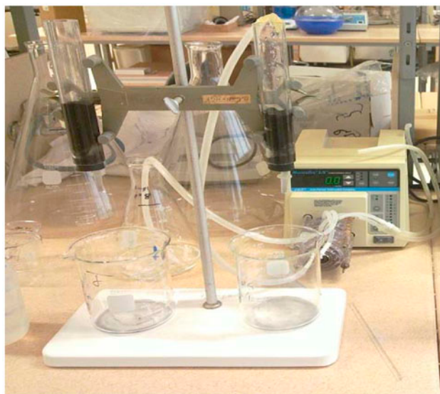
Fig. 1. View of the experimental setup for fixed-bed adsorption columns.
