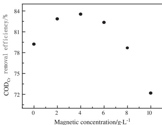
Fig. 3. The removal efficiency of COD<sub>Cr</sub> at different magnetic powder dosage.
