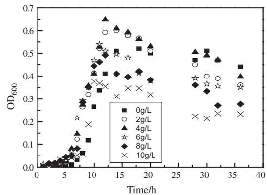
Fig. 2. The growth curves of microorganisms at different magnetic powder dosage.
