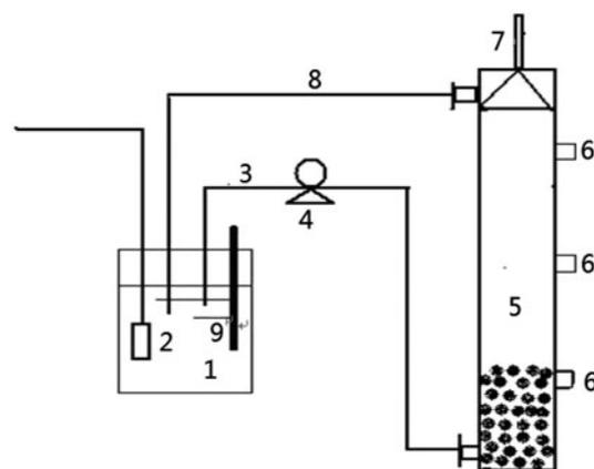
Fig. 1. Experimental equipment diagram. (1) Aeration tank; (2) air diffuser ball; (3) inlet pipe; (4) pump; (5) reactor; (6) sampling valve; (7) three-phase separator; (8) effluent pipe; (9) heater.
