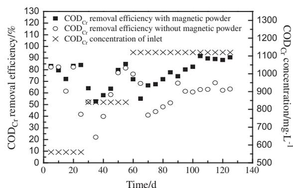
Fig. 4. Changes of COD<sub>Cr</sub> removal efficiency during cultivation.
