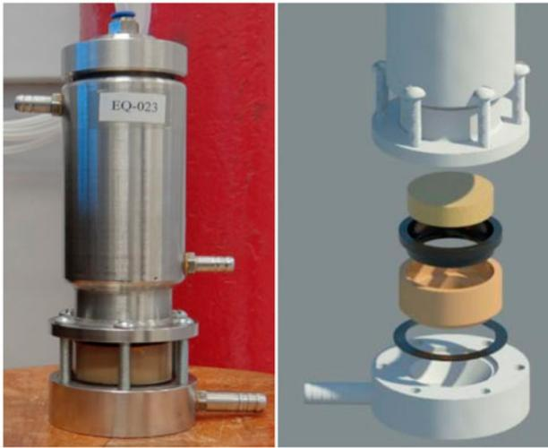
Fig. 7. Filter pilot for the dead-end filtration.
