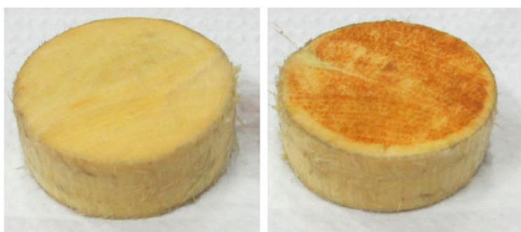
Fig. 17. Caixeta samples before and after the dead-end filtration.
