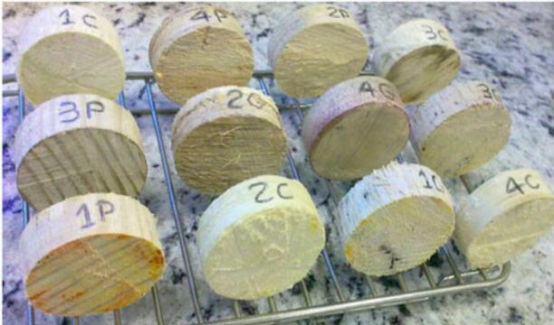
Fig. 6. Filter elements for the dead-end filtration.
