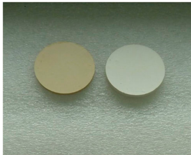
Fig. 5. Diatomite porous ceramic membrane (a) after filtration and (b) before filtration.
