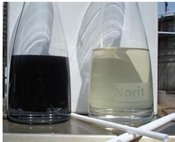
Fig. 6. Comparison of the effluents qualities: (left) UASB and (right) AnMBR pilot.
