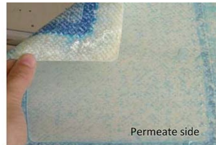
Photograph 21.- Methylene blue test massive positive result
