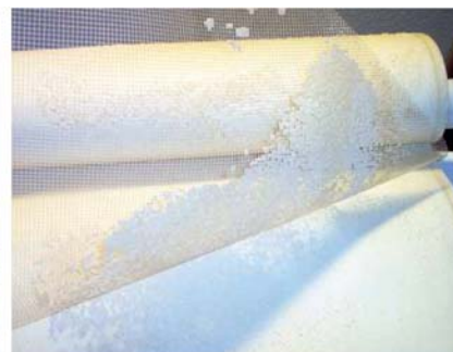
Photograph 18.- Calcium Sulphate scale on spacer
