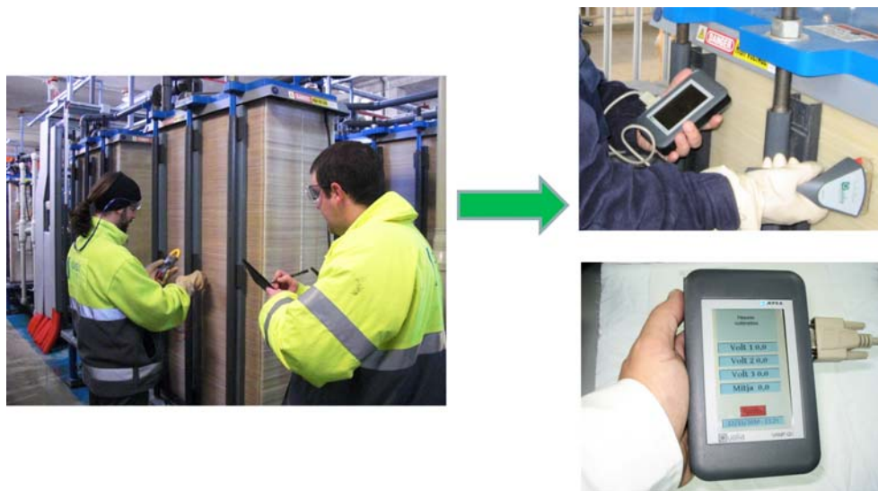
Fig. 1. Stack probing evolution procedure. From manual to semi-automated work, using the new equipment developed by the R&D Department (ATLL, patent pending).
