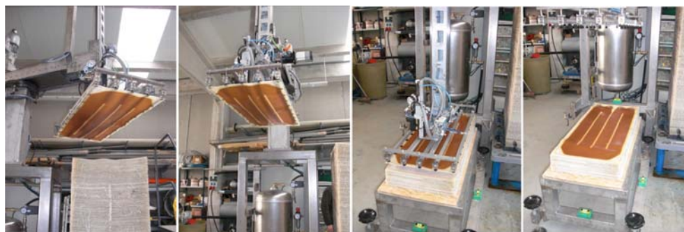
Fig. 3. Robotic device for assembly and disassembly the EDR stack.
