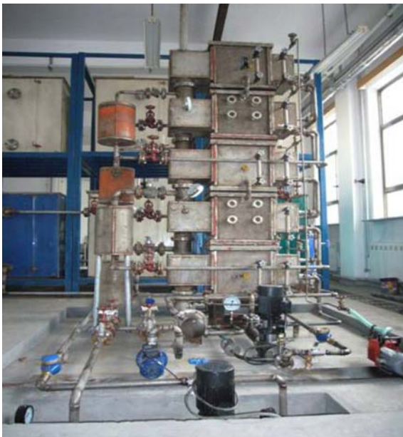
Fig. 2. Picture of the experimental five-effect distillation desalination setup.
