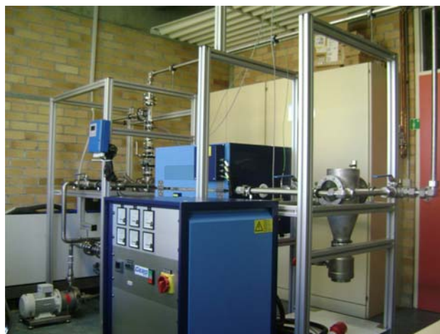
Fig. 1. Fouling test rig equipped with projectile injection system.
