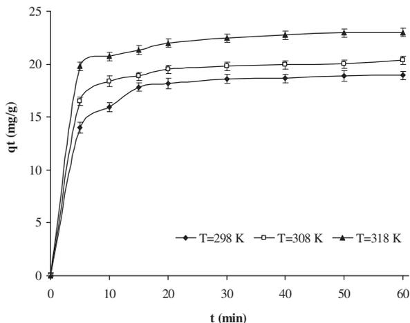
Fig. 1(a). Effect of contact time on the adsorption of MB on *B. subtilis* at different temperatures ( $V=100\text{ mL}$ ,  $m=0.1\text{ g}$ , agitation speed = 150 rpm, initial concentration = 50  $\text{mg L}^{-1}$ ). The experiments and measurements were performed in three independently replicates. Confidence intervals of 95% were calculated for the data ( $n=3$ ) and error bars represent standard deviations.
