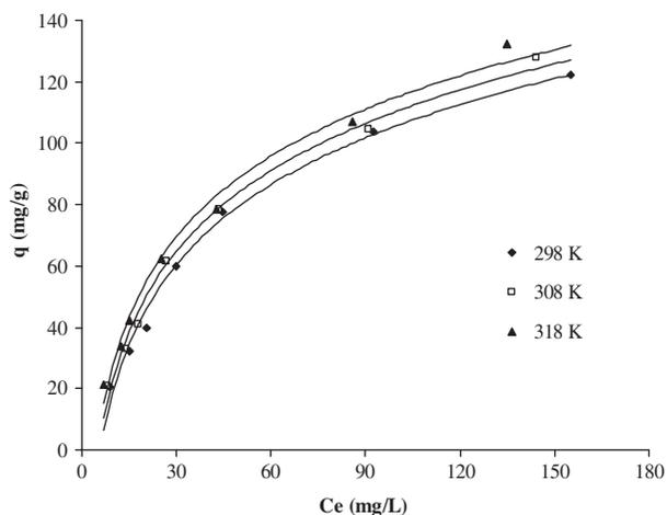
Fig. 2. Adsorption isotherms of MB on *B. subtilis* at different temperatures.
