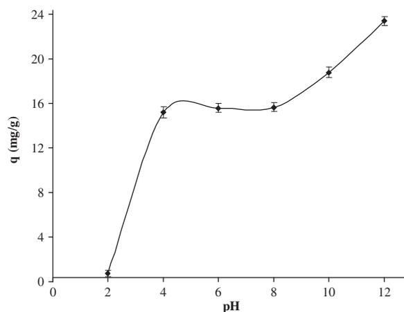
Fig. 3. Effect of pH on the adsorption of MB on *B. subtilis* ( $V = 100$  mL,  $m = 0.1$  g, agitation speed = 150 rpm, initial concentration =  $50 mg L^{-1}$ ). The experiments and measurements were performed in three independently replicates. Confidence intervals of 95% were calculated for the data ( $n = 3$ ) and error bars represent standard deviations.
