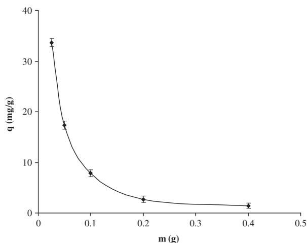
Fig. 4. Effect of adsorbent dose on initial adsorption rates ( $V = 100$  mL, agitation speed = 150 rpm, temperature = 298 K, pH = 6.0). The experiments and measurements were performed in three independently replicates. Confidence intervals of 95% were calculated for the data ( $n = 3$ ) and error bars represent standard deviations.
