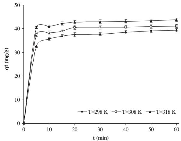
Fig. 1(b). Effect of contact time on the adsorption of MB on *B. subtilis* at different temperatures ( $V=100\text{ mL}$ ,  $m=0.1\text{ g}$ , agitation speed = 150 rpm, initial concentration = 100  $\text{mg L}^{-1}$ ). The experiments and measurements were performed in three independently replicates. Confidence intervals of 95% were calculated for the data ( $n=3$ ) and error bars represent standard deviations.
