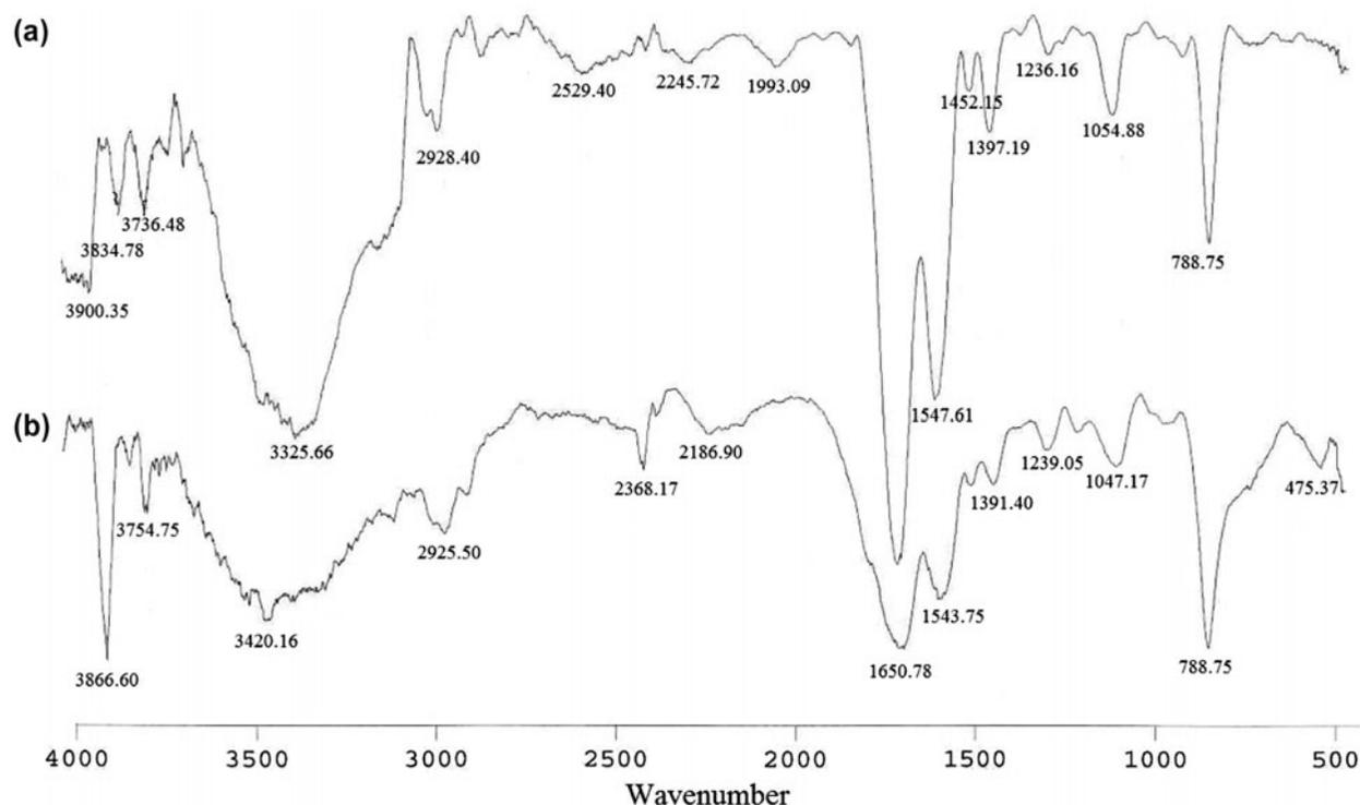
Fig. 5. FTIR spectra of *B. subtilis* (a) before MB was loaded and (b) after MB was loaded.
