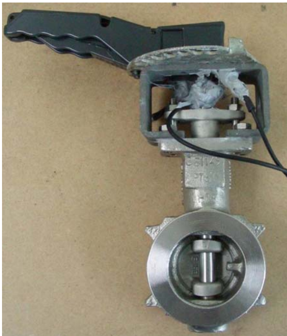
Fig. 15. Photograph of the 316L butterfly valve before exposure.
