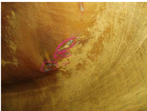
Fig. 5. Pitting corrosion of the casing of a HP booster pump (cast duplex stainless steel UNS J93550, DIN 1.4468).
