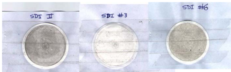
Fig. 4. SDI test membrane operated on UF permeate.
