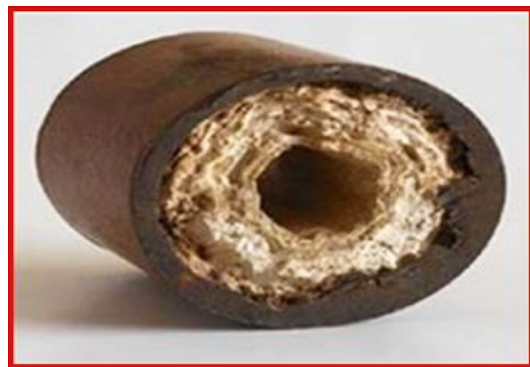
Fig. 2. A scaled household water pipe.
