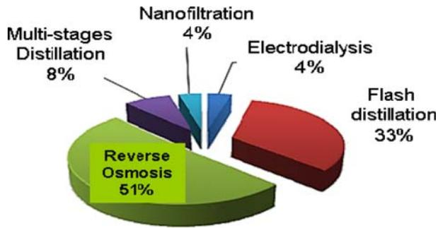
Fig. 1. Installed plant in the world for water desalination technics.
