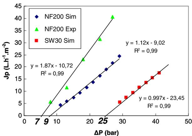
Fig. 9. Permeate flow vs. transmembrane pressure for NF200 experiments with natural seawater and simulation in comparison with simulation of the SW30.
