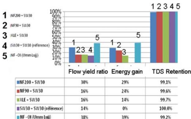
Fig. 14. Flow yield ratio, energy gains, and TDS retention for the different studied configurations.
