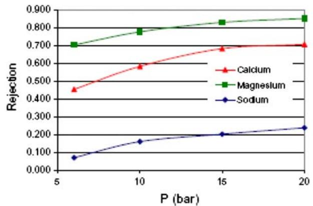
Fig. 6. Monovalent/divalent ions selectivity in NF70 membrane seawater (from Pontić et al. [4]).
