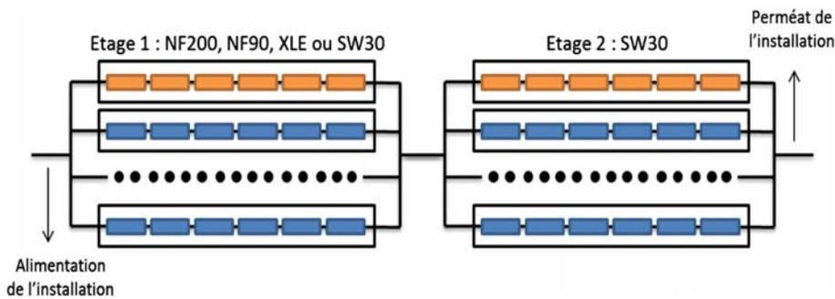
Fig. 13. Design of Umm Lujj stages 1 and 2.
