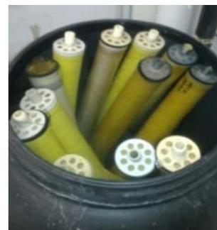
Fig. 3. Membranes modules 2,540 stocked in 1% sodium bisulfite solution (photography J.-S. Derauw, 05/04/2011).
