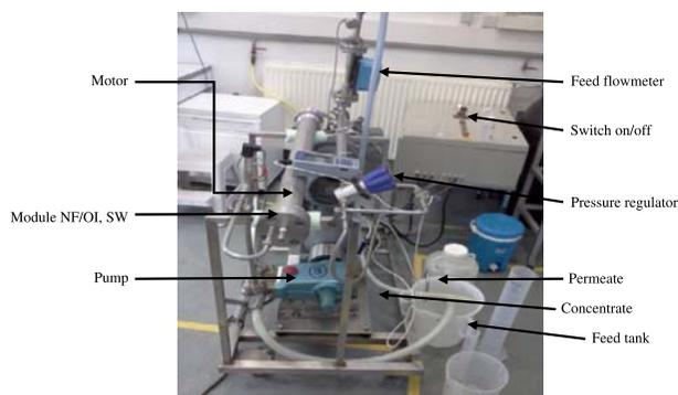
Fig. 2. Pilot for laboratory scale experiments equipped with membrane module 25–40.
