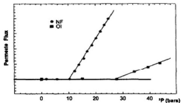
Fig. 5. Comparison of NF and RO permeability to seawater (from Pontié et al. [3]) NF90 and ESPA3 membranes.
