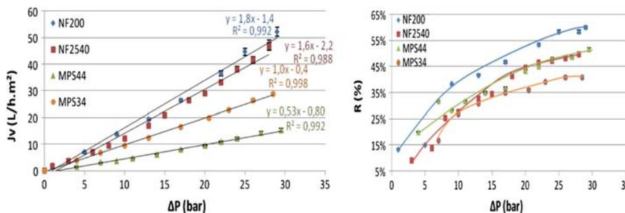
Fig. 7.  $J_v = f(\Delta P)$  and  $R = f(DP)$  for the studied membranes (NaCl 35 g/L, feed flow 600 L/h, temperature 20 °C, flow yield ratio 1–10%, module 2,540 (membrane area 2.6 m<sup>2</sup>)).
