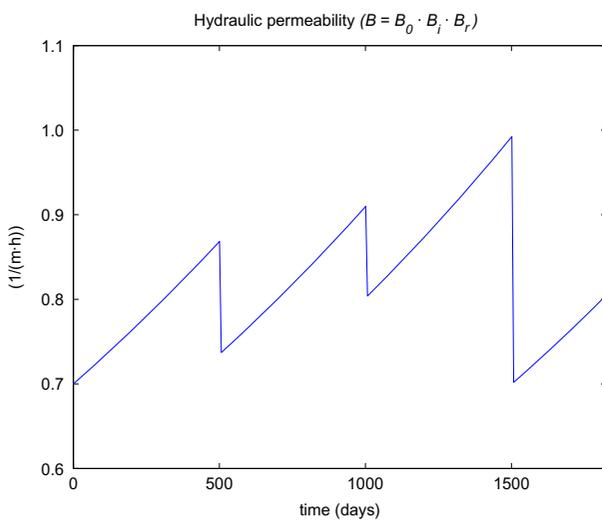
Fig. 7. Total salt permeability over five years, with a chemical cleaning at 500 days, partial replacement at 1,000 days, and full replacement of the modules at 1,500 days.
