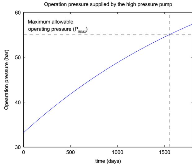
Fig. 2. Operation pressure. Maximum value of 55 bar exceeded after 1,550 days.
