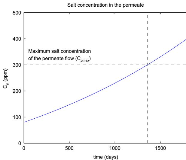
Fig. 3. Salt concentration of the permeate flow. Maximum value of 300 ppm exceeded after 1,350 days.
