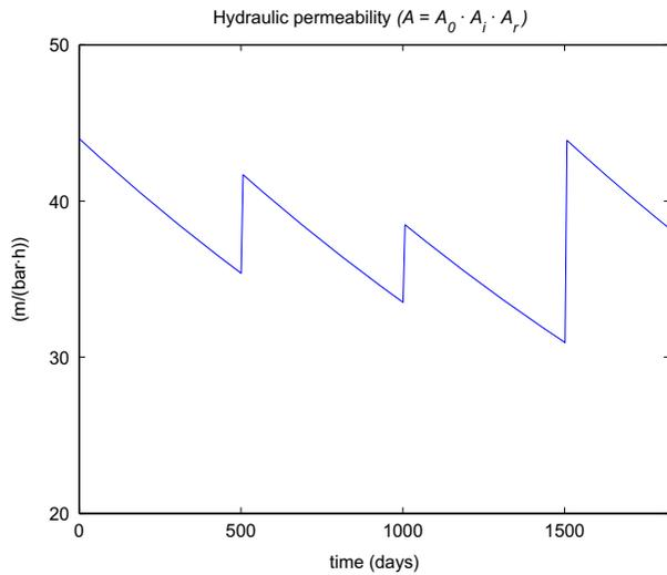
Fig. 6. Total hydraulic permeability over five years, with a chemical cleaning at 500 days, partial replacement at 1,000 days, and full replacement of the modules at 1,500 days.
