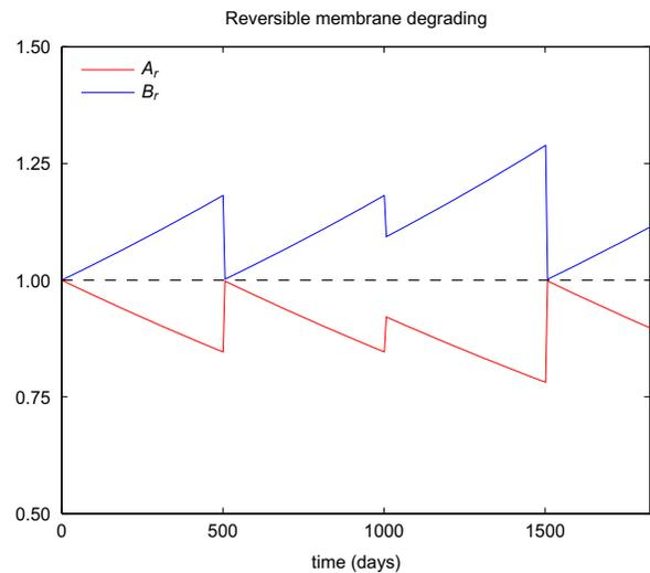
Fig. 5. Reversible factor for the hydraulic and salt permeabilities.
