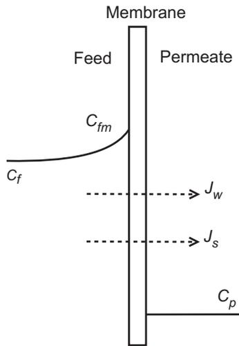
Fig. 1. Salt concentration gradient on both sides of the membrane.
