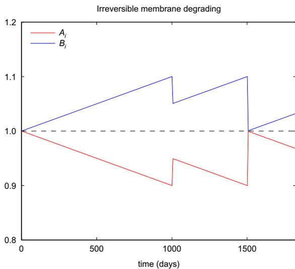
Fig. 4. Irreversible factor for the hydraulic and salt permeability.
