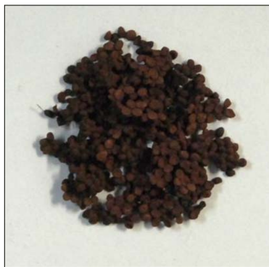
Fig. 2. Alginate/PVA-hematite composite used in the experiments.
