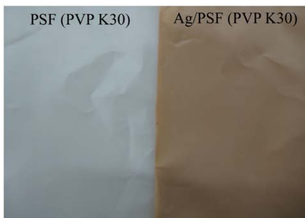
Fig. 2. Macroscopic morphologies of PSF (PVP K30) and Ag/PSF (PVP K30) composite membranes.
