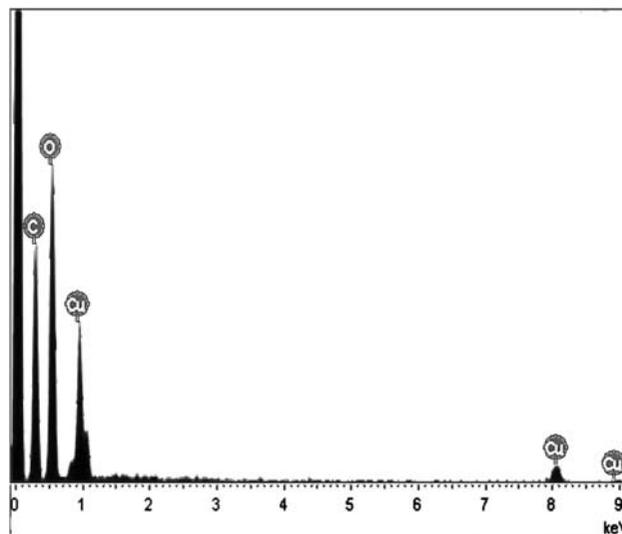
Fig. 6. EDS spectrum of Cu(II)-loaded 110 resin.
