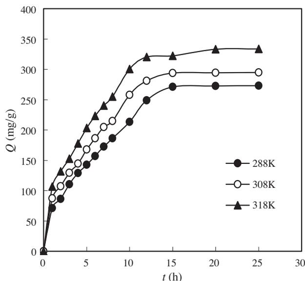
Fig. 2. Adsorption amount of different temperatures, resin 20.0 mg,  $[Cu^{2+}]_0 = 0.34$  mg/mL, pH = 5.28, 100 rpm.
