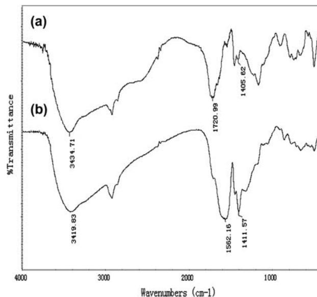
Fig. 4. IR spectra of 110 resin (a) before and (b) after loaded Cu(II).
