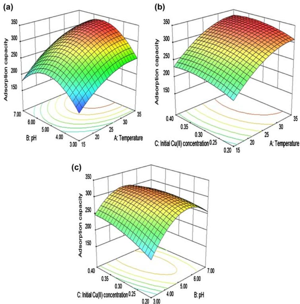
Fig. 1. Three-dimensional plots showing effects of (a) pH and temperature, (b) temperature and initial Cu(II) concentration, and (c) pH with initial Cu(II) concentration interactions on adsorption capacity of 110 resin for Cu(II).
