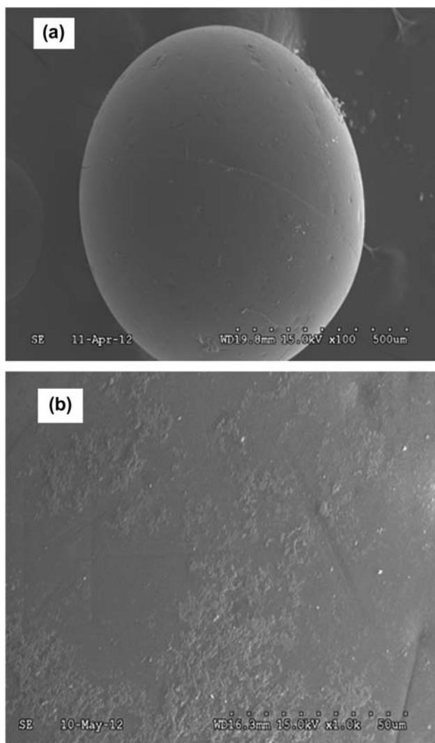
Fig. 5. SEM images of (a) dried unloaded 110 resin and (b) Cu(II)-loaded 110 resin.
