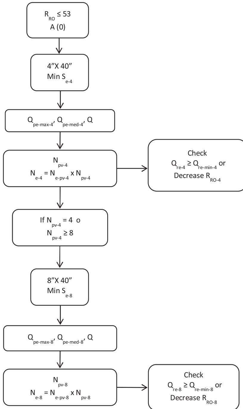
Fig. 6. RO system checks and settings ( $R_{RO} \leq 53\%$ ).
