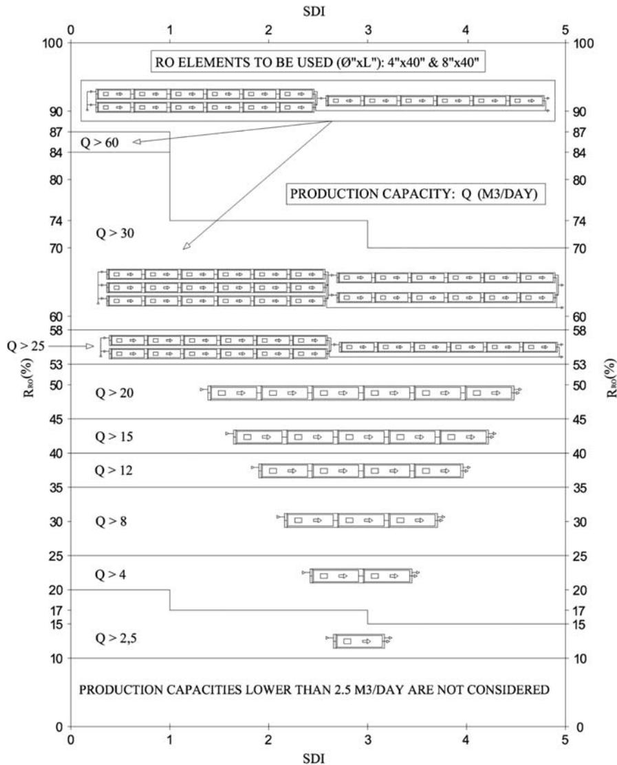
Fig. 3. Basic arrangement and production capacity distribution.
