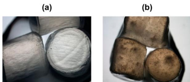
Fig. 2. Images of Biocontact N biocarrier: as received (a) and after inoculation (b) at 25 $\times$  magnification.
