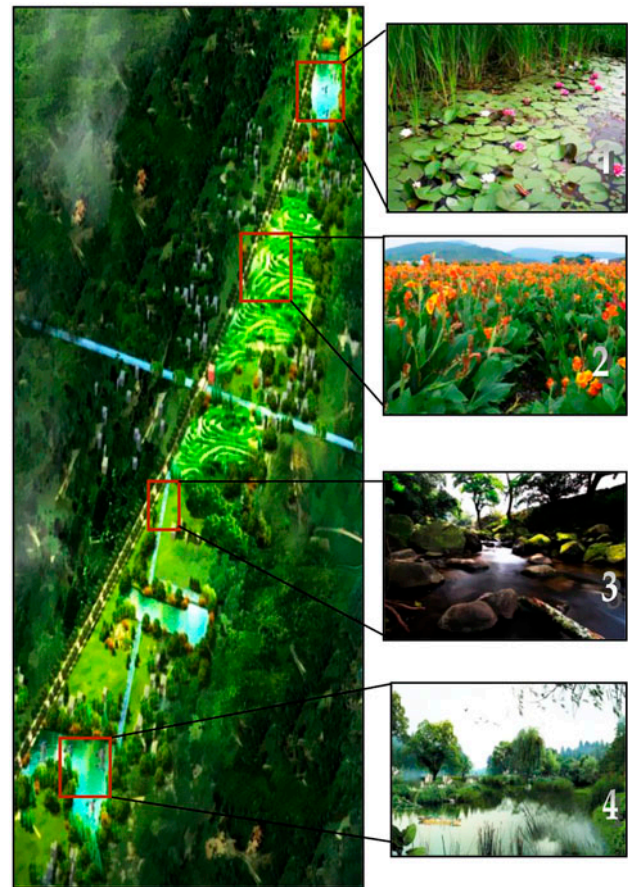
Fig. 4. The bird's eye view of this whole system. (1) Stabilization pond; (2) free water system wetland; (3) ecotype corridor; (4) retention facility.
