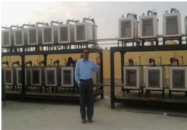
(a) Photo of double deck MSF desalination test pilot unit
