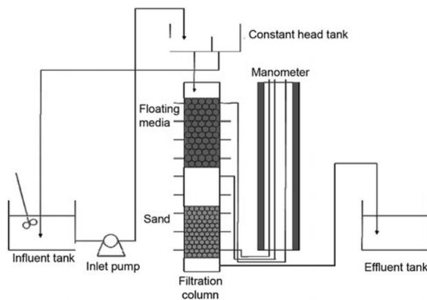
Fig. 1. Apparatus of filtration system.
