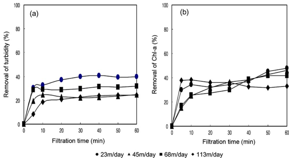
Fig. 5. Removal of (a) Turbidity and (b) Chl-a at the different velocity.
