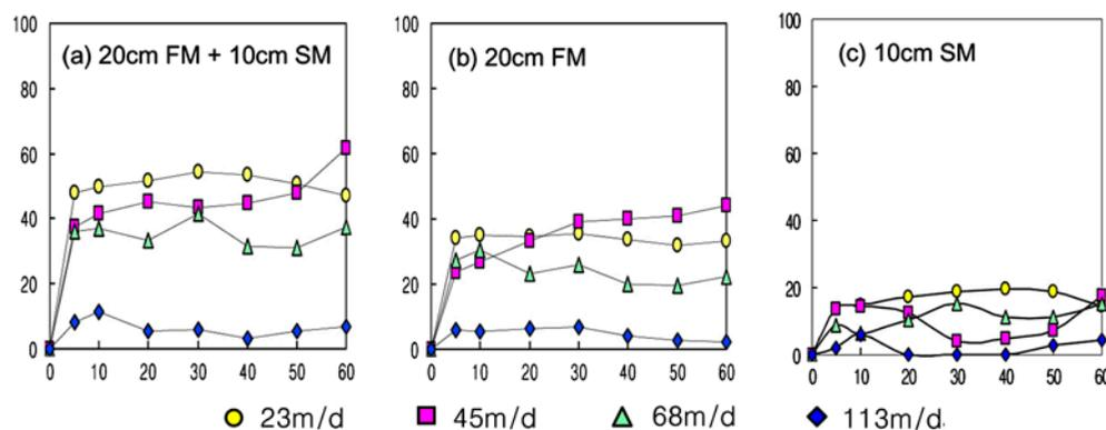
Fig. 3. Removal of MA at various filtration velocities (initial cell number:  $4.52 \times 10^4$  cells/ml).
