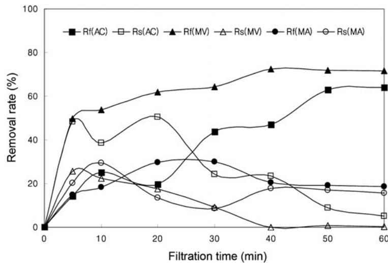
Fig. 2. Removal rate of three algae with filtration time (initial cell number:  $8.29 \times 10^4$  cells/ml).
