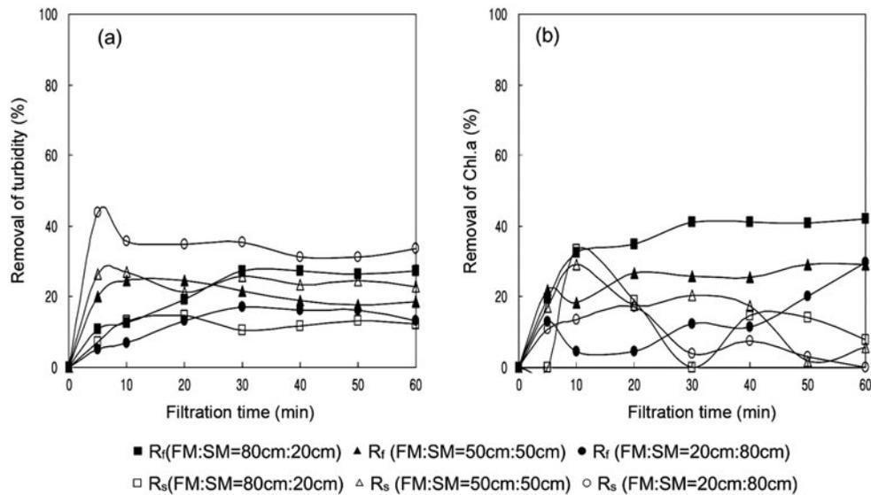
Fig. 4. Removal of (a) Turbidity and (b) Chl-a by various depths of dual media.
