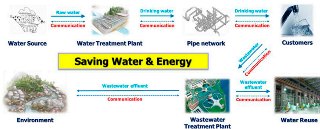
Fig. 1. Smart water grid: Water network with communication to save water and energy.
