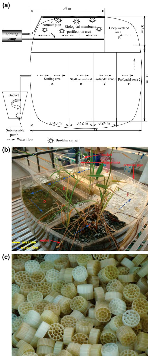
Fig. 1. (a) Schematic diagram and actual photograph of the pre-dam, (b) Actual photograph of the pre-dam, (c) Ackermann packing.
