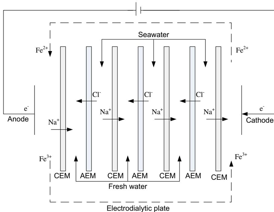
Fig. 6. Removal of charged ions in a reverse electrodialysis set-up (image adapted from Fernando) [45].
