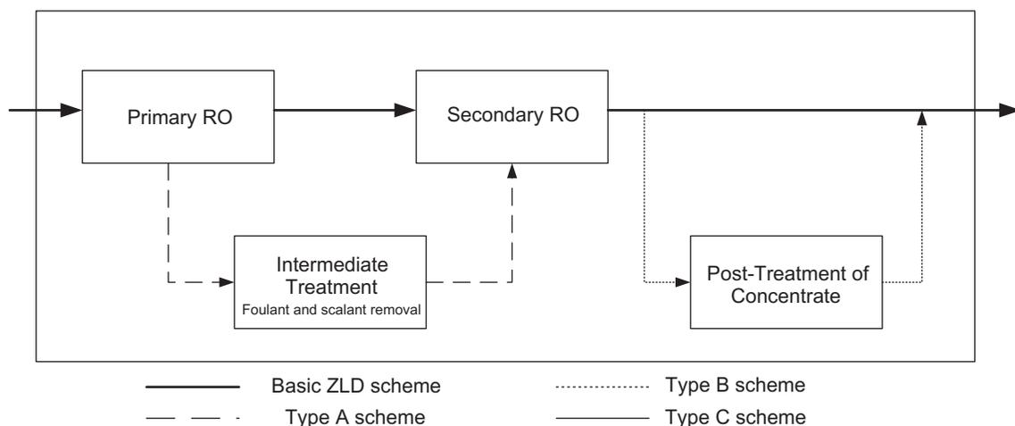
Fig. 5. The ZLD classification scheme (adapted from Perez-Gonzalez et al.) [42].
