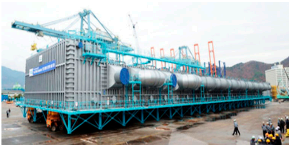
Fig. 1(a). One of 8 MSF units at Ras Al Khair plant, SA. of $US1.76 billion total cost billion, capacity/unit = 91,000 t/d (20 MIGD) or $11 M/MIGD, 123 m (l) × 33.7 m (w), and 4,150 t [3].
