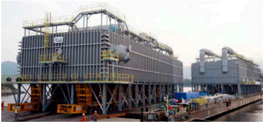
Fig. 24(b). Marafic Yanbu 2 \times 6.07 MIGD ME-TVC units having rectangular vessel along the TC, shipped on 29 July 2012, from DOOSAN.
