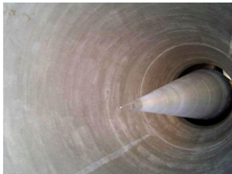
Fig. 25(b). The TC used in ME-TVC with moving nozzle [18].
