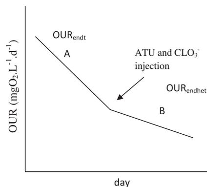
Fig. 2. Respirometric tests obtained after punctual addition of ATU and ClO<sub>3</sub><sup>-</sup> inhibitor.
