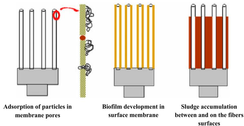
Fig. 3. Fouling mechanisms development in hollow fiber membrane.
