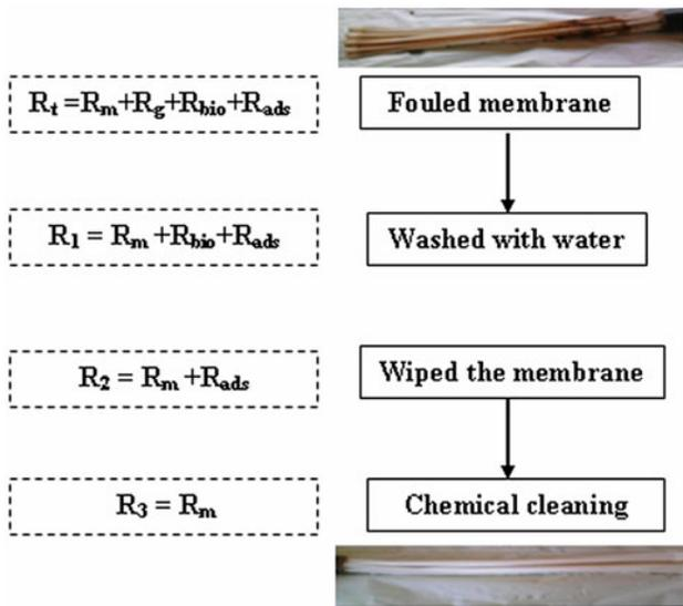
Fig. 4. Procedure of membrane cleaning.
