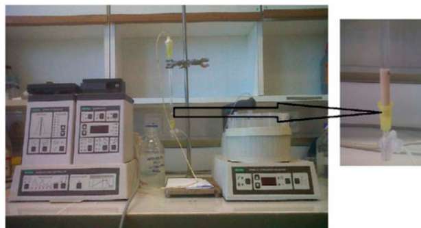
Fig. 2. System for continuous elimination of MPs, equipped with 3.5 \times 0.7 cm column packed with laccase immobilized on CPC beads.
