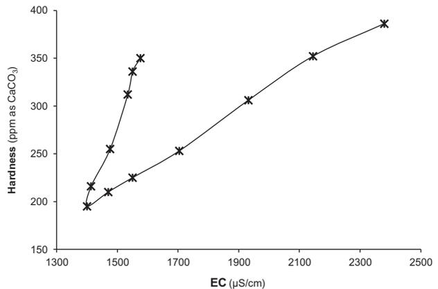
Fig. 6. Changes in hardness as a function of EC for a typical water in a lime treated jar test.
