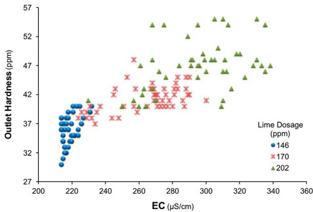
Fig. 7. Outlet hardness as a function of EC of treated water in ESP lime softening clarifier.
