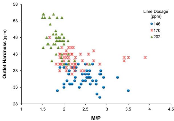
Fig. 3. Change of hardness of treated water at various lime dosages versus *M* and *P* alkalinity ratio.
