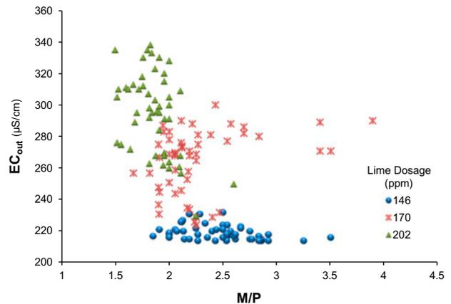
Fig. 5. Outlet EC as a function of *M* and *P* alkalinity ratio of the treated water at various lime dosages.
