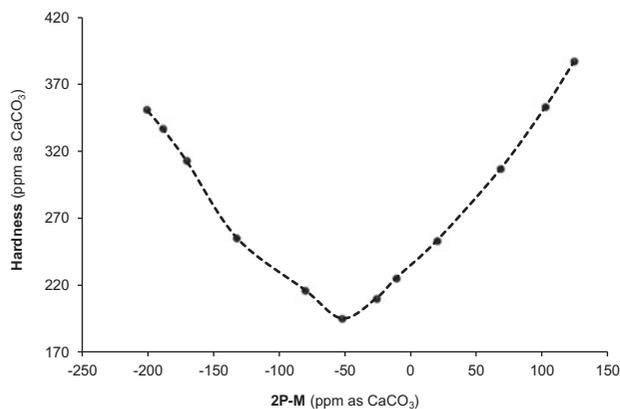
Fig. 1. Changes in hardness and  $(2P-M)$  of a typical softened water in a lime treated jar test.
