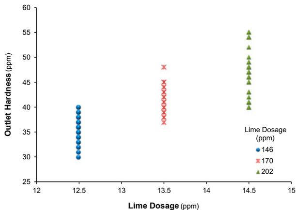
Fig. 4. Change of outlet hardness versus lime dosage.
