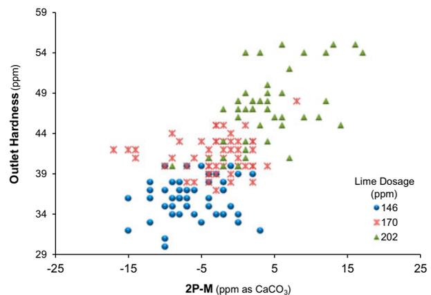
Fig. 2. Change of hardness versus  $(2P-M)$  of treated water at various lime dosages.
