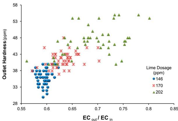
Fig. 8. Changes in outlet hardness as a function of the ratio of the ECs of outlet and inlet water in various lime dosages in ESP lime softening clarifier.
