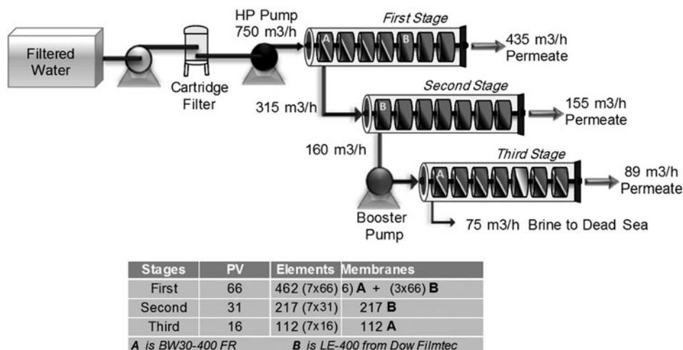
Fig. 4. RO skid configuration.
