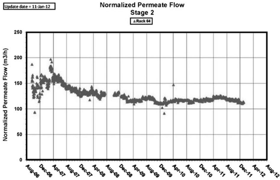
Fig. 12. Second stage normalized permeate flow.
