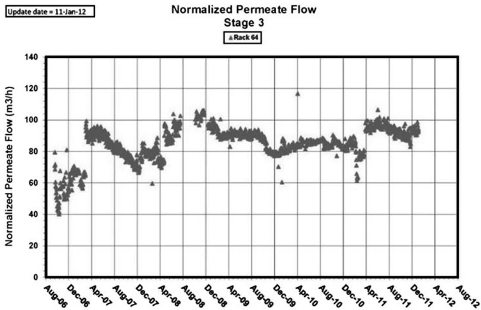
Fig. 13. Third stage normalized permeate flow.
