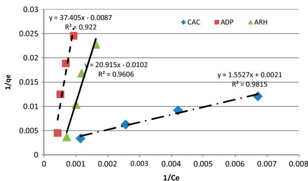
Fig. 6. Langmuir isotherm for COD reduction onto ADP, ARH, and CAC.
