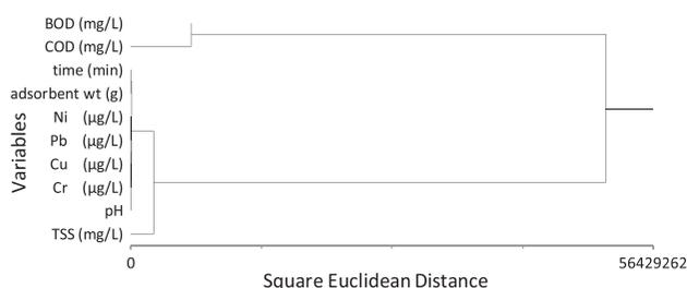
Fig. 5. Dendrogram depicts the relationship between reduced treated effluent main parameters and the optimum adsorbent dose (CAC, ARH, and ADP), contact time, and solution pH using Ward's methods for minimum variance.
