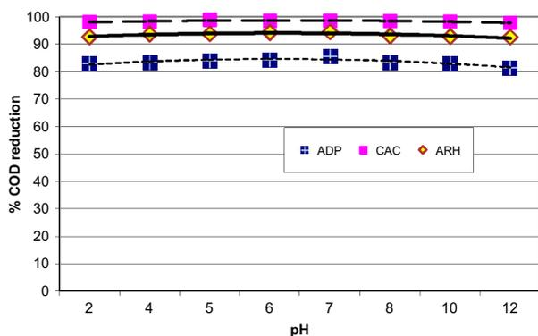
Fig. 4. The effect of varying pH upon % COD reduction, adsorbent weights (100 g/L AC, 180 g/L ARH and 120 g/L ADP), time = 120 min,  $T=25^{\circ}\text{C}$ , volume of solution 50 mL, and  $\text{COD}_0=6,760\text{ mg/L}$ .
