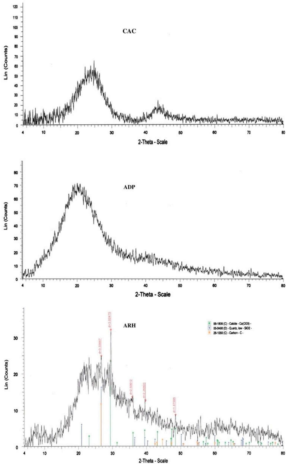
Fig. 1. X-ray diffraction (XRD) spectra of commercial activated carbon (CAC), activated date pits (ADP) and activated rice husks (ARH).
