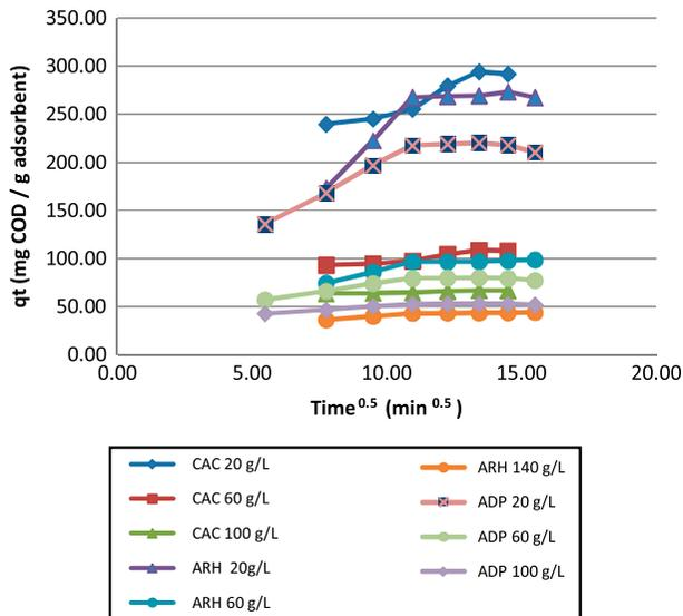
Fig. 8. Intraparticle diffusion model for adsorption/reduction of COD onto CAC, ARH, and ADP.  $T = 25^{\circ}\text{C}$ , volume of solution 50 mL, and  $\text{COD}_0 = 6,760 \text{ mg/L}$ .
