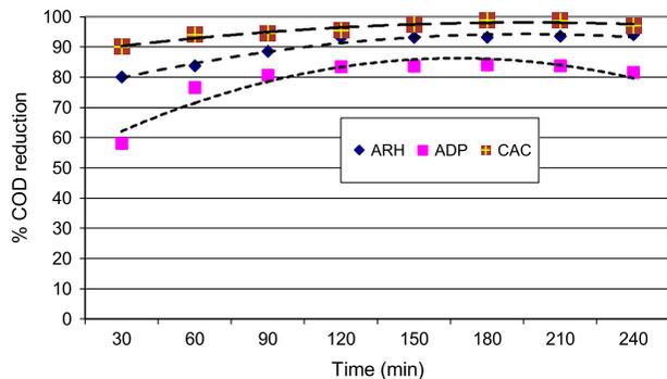
Fig. 3. The effect of varying the stirring/ contact time (min) upon % COD reduction at pH 7, adsorbent weights (100 g/L CAC, 180 g/L ARH and 120 g/L ADP),  $T=25^{\circ}\text{C}$ , volume of solution 50 mL, and  $\text{COD}_0=6,760\text{ mg/L}$ .
