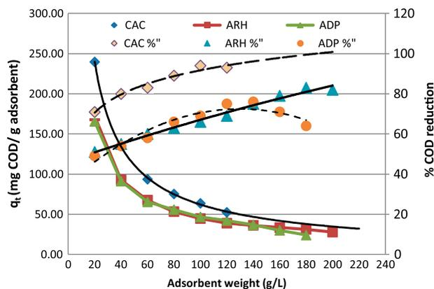
Fig. 2. The effect of adsorbent weight (ADP, ARH and CAC) upon % COD reduction and  $q_t$  (mg COD/g adsorbent) at pH 7;  $t_{CAC} = 120$  min,  $t_{ADP} = 120$  min and  $t_{ARH} = 120$  min;  $T = 25$  °C, volume of solution 50 mL, and  $COD_0 = 6,760$  mg/L.
