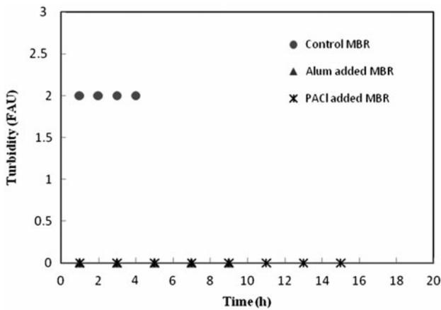
Fig. 7. Permeate turbidity in three MBRs during their operations.
