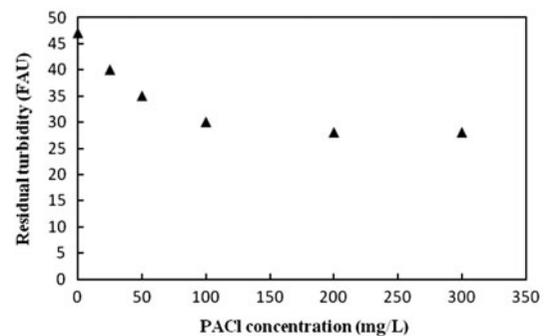
Fig. 3. Residual turbidity in different concentration of PACl.
