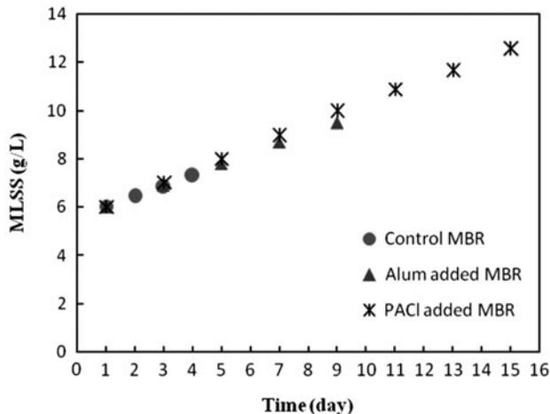
Fig. 9. MLSS concentration in control and flocculant-added MBRs.
