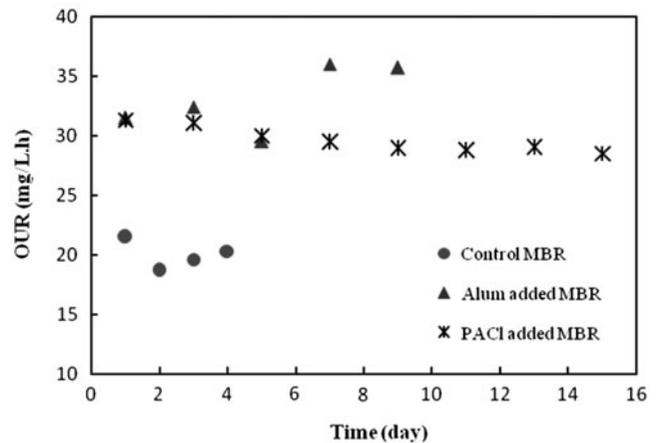
Fig. 8. Activated sludge OUR in control and flocculant-added MBRs.
