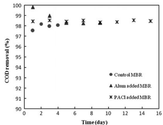
Fig. 5. COD removal in control and flocculant-added MBR.
