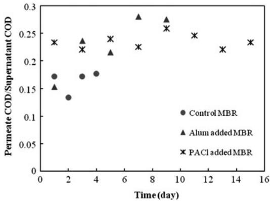
Fig. 6. Permeate COD to supernatant COD ratio in three MBRs.
