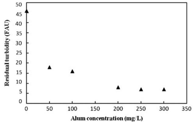
Fig. 2. Residual turbidity in different concentration of alum.
