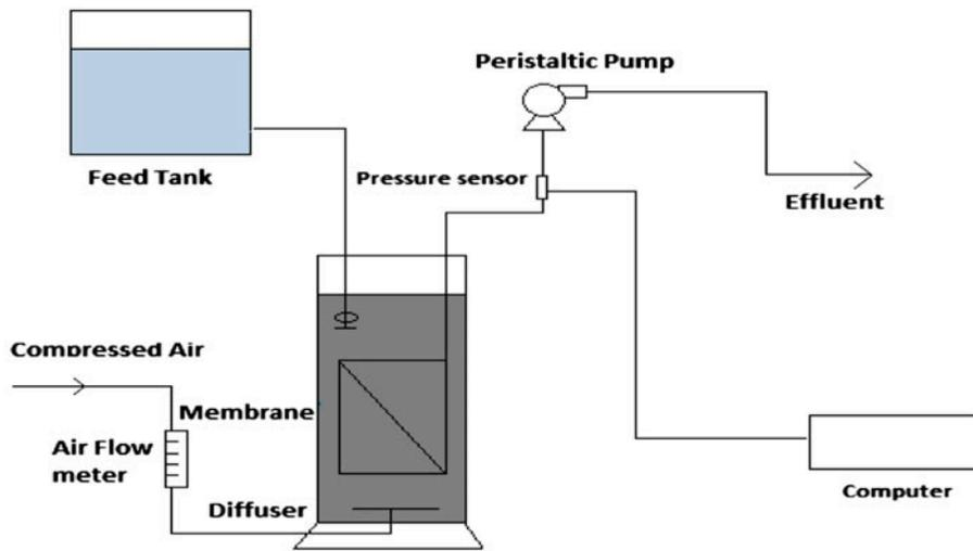
Fig. 1. Schematic diagram of the membrane bioreactor system.
