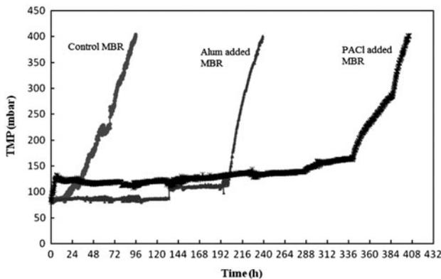
Fig. 4. TMP profile of control and flocculant-added MBRs.
