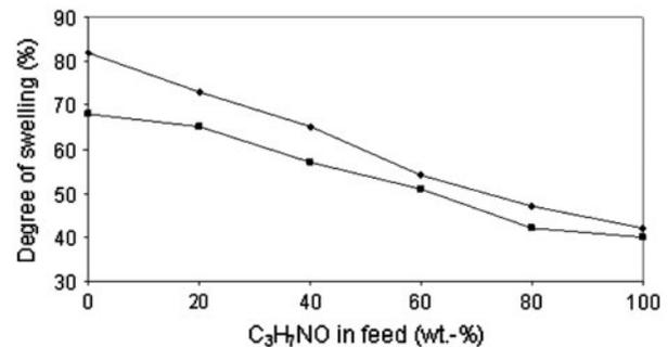
Fig. 4. Change in the swelling degree with the feed composition. (◆: NaAlg in liquid; ■: NaAlg in vapour).
