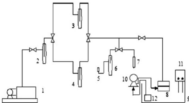
Fig. 2. Schematic diagram of the pervaporation apparatus: (1) vacuum pump, (2–4, 6) permeation traps; (5) McLeod manometer; (7) vent; (8) permeation cell; (9) constant temperature water bath; (10) peristaltic pump; and (11) temperature indicator.
