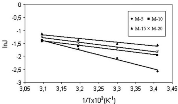
Fig. 10. In VP method, variation of  $\ln J$  with temperature for different membranes at 20 wt.% of DMF in the feed. ( $\circ$ : M-5;  $\square$ : M-10;  $\triangle$ : M-15;  $\times$ : M-20).
