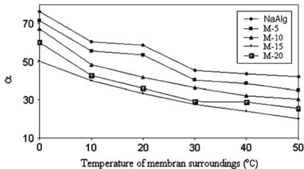
Fig. 14. Effect of membrane surroundings temperature on the separation factor. The permeation conditions;  $P$ : 0.5 mbar, temperature of feed solution ( $t$ ): 40°C.
