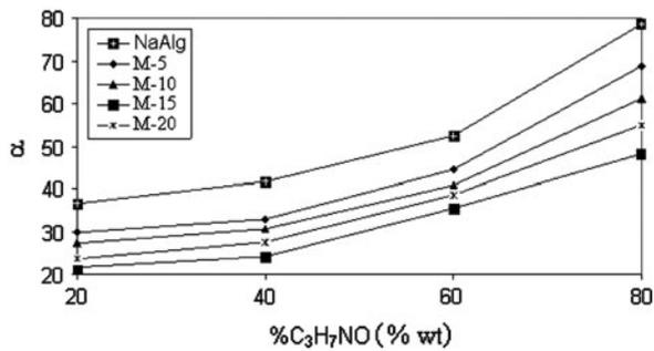
Fig. 12. Change of separation factor with the feed vapor composition in TDVP. The permeation conditions; temperature of membrane surroundings: 15°C,  $P$ : 0.5 mbar, temperature of feed solution ( $t$ ): 40°C.
