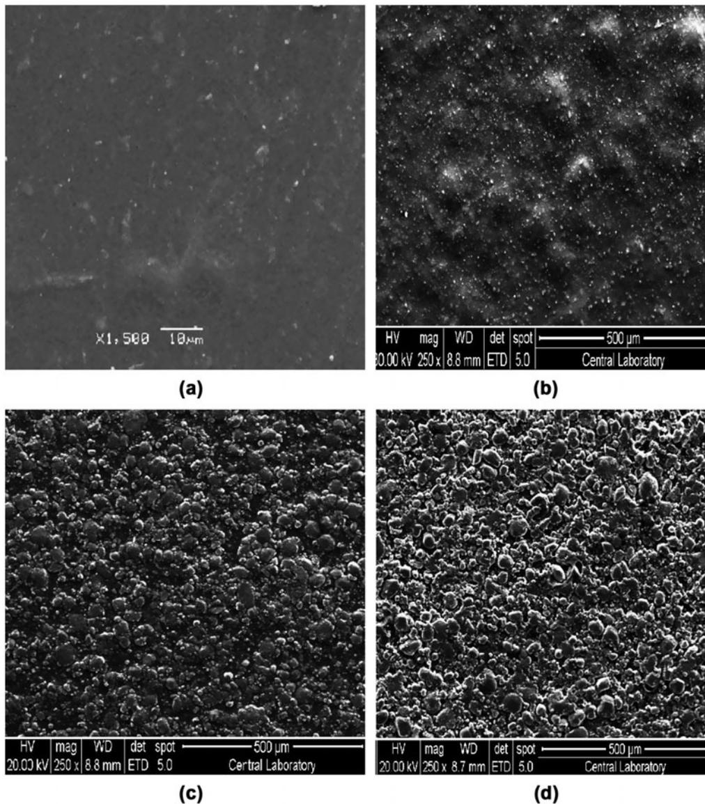
Fig. 3. Scanning electron microscopic picture of (a) pristine NaAlg membrane (b,c,d) NaAlg/Clt (5,10,15 wt.%, respectively) composite membrane (Ref. [33]).
