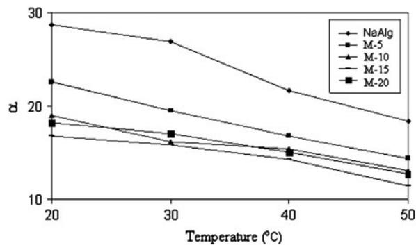
Fig. 9. Effect of temperature on selectivity in VP. The permeation conditions; DMF: 20 wt.%,  $l$ : 60  $\mu$ m,  $P$ : 0.5 mbar.
