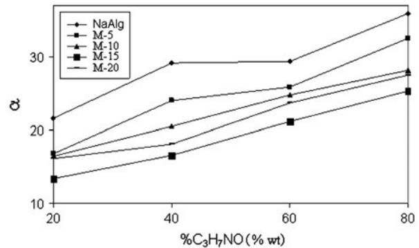
Fig. 7. Variation of selectivity with feed vapor concentration for pristine NaAlg and NaAlg/Clt membranes in VP. The permeation conditions;  $l$ : 60  $\mu$ m,  $t$ : 40°C,  $P$ : 0.5 mbar.
