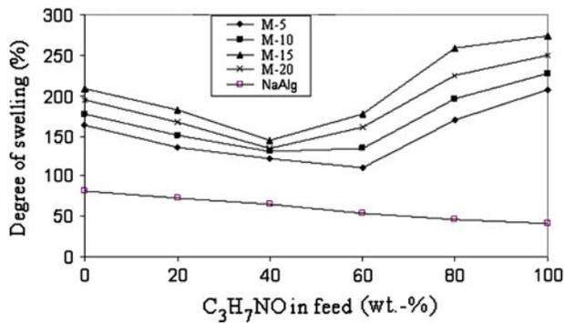
Fig. 5. Variation of degree of swelling with different wt.% of Clt for 20 wt.% of DMF in the feed.
