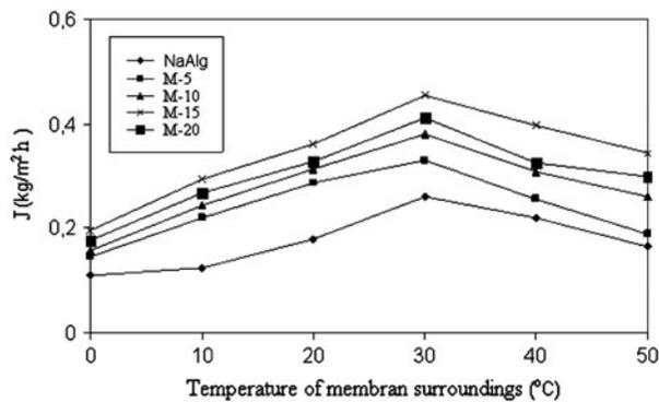
Fig. 13. Effect of membrane surroundings temperature on the permeation rate. The permeation conditions;  $\lambda$ : 60  $\mu\text{m}$ ,  $P$ : 0.5 mbar, temperature of feed solution ( $t$ ): 40°C.
