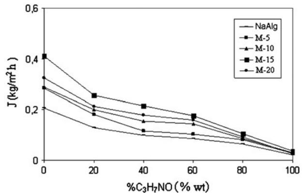
Fig. 6. Variation of flux with feed vapor concentration for pristine NaAlg and NaAlg/Clt membranes in VP. The permeation conditions;  $l$ : 60  $\mu$ m,  $t$ : 40°C,  $P$ : 0.5 mbar.
