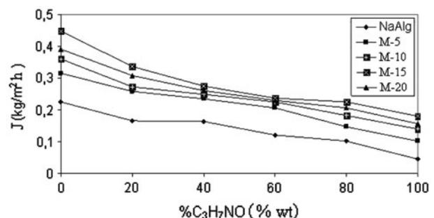
Fig. 11. Change of permeation rate with the feed vapor composition in TDVP. The permeation conditions; temperature of membrane surroundings: 15°C,  $P$ : 0.5 mbar, temperature of feed solution ( $t$ ): 40°C.
