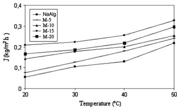
Fig. 8. Effect of temperature on flux in VP. The permeation conditions; DMF: 20 wt.%,  $l$ : 60  $\mu$ m,  $P$ : 0.5 mbar.
