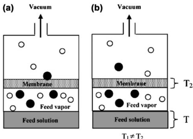
Fig. 1. Principal schemes of (a) the VP and (b) the TDVP cells.
