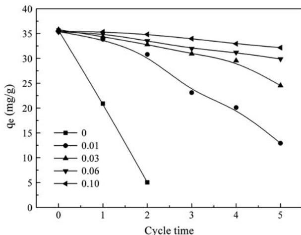
Fig. 3. Variations of adsorption capacities with cycle times under different NaOH concentration in eluent.
