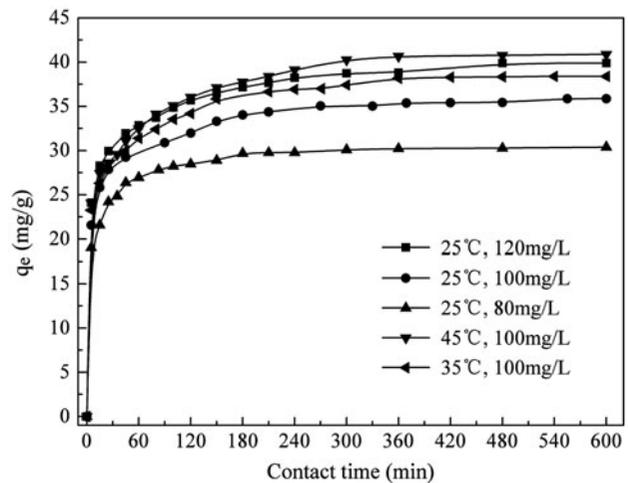
Fig. 1. Effect of contact time on CR adsorption onto PLR.
