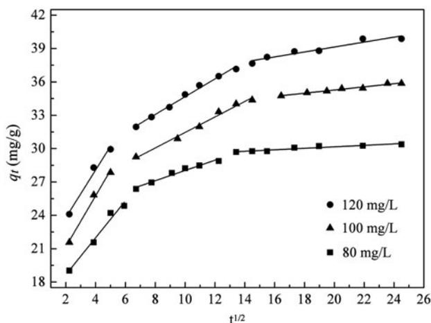
Fig. 2. Intra-particle diffusion plots for CR adsorption onto PLR.
