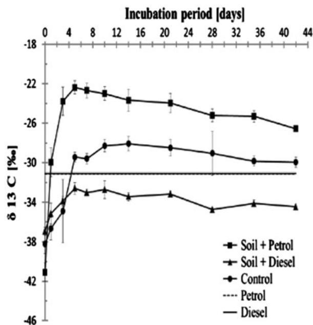
Fig. 2. Values of  $\delta^{13}C$  in the samples in successive incubation days and substrate delta. Straight lines represent  $\delta^{13}C$  of pure substrates (Table 2): the continuous line denotes diesel oil, and the dashed line represents petrol (mean values  $\pm$  SE).
