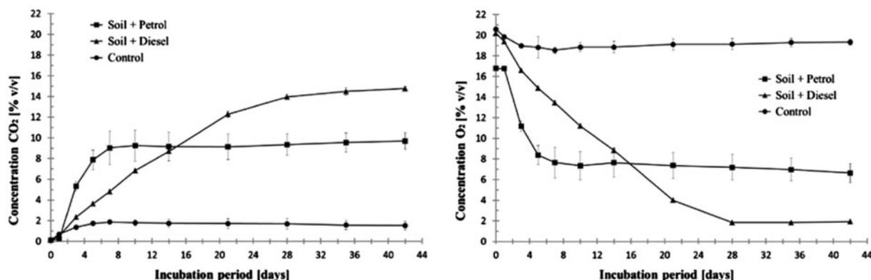
Fig. 1. Changes in the gas concentration in the headspace over soil contaminated with petroleum derivatives during successive days of incubation: (a)  $\text{CO}_2$ ; (b)  $\text{O}_2$  (mean values  $\pm$  SE).
