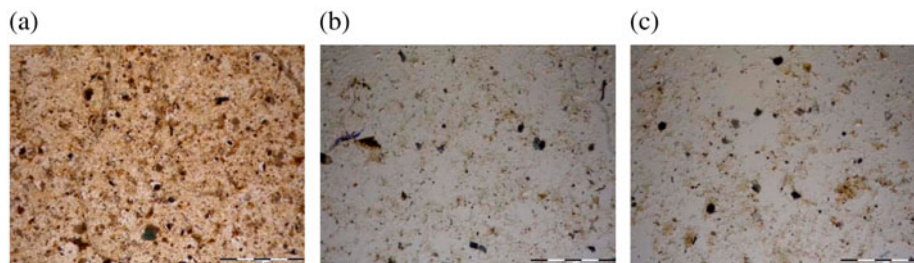
Fig. 4. The structure of non-prepared sewage sludge submitted anaerobic stabilization, (a) 0 d of fermentation, (b) 5 d of fermentation and (c) 10 d of fermentation.
