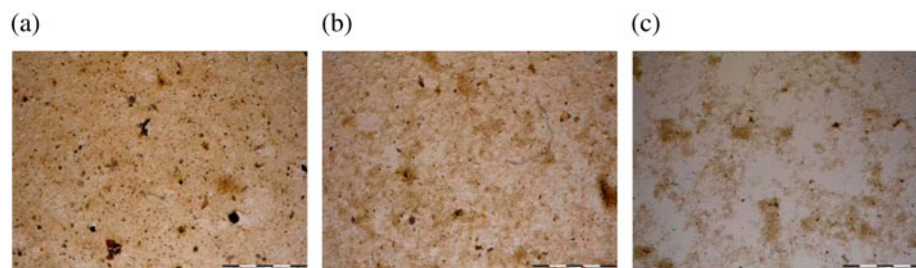
Fig. 7. The structure of ultrasonic conditioned sewage sludge submitted anaerobic stabilization, (a) 0 d of fermentation, (b) 5 d of fermentation and (c) 10 d of fermentation.
