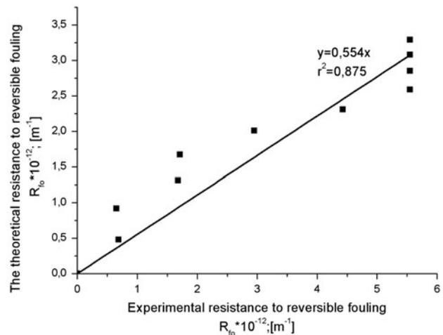
Fig. 5. Comparison of changes in resistance of the  $R_{\text{rev. exp.}}$  polysulfone membrane during the post-process coke wastewater ultrafiltration treatment.
