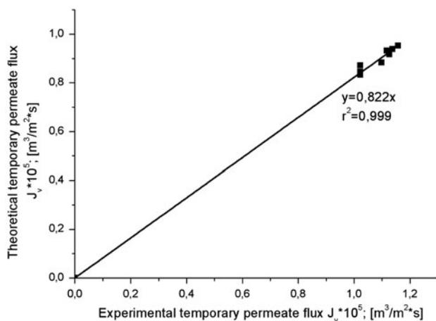
Fig. 7. Comparison between theoretical permeate flux calculated from the hydraulic resistance model and the size of temporary stream determined experimentally.
