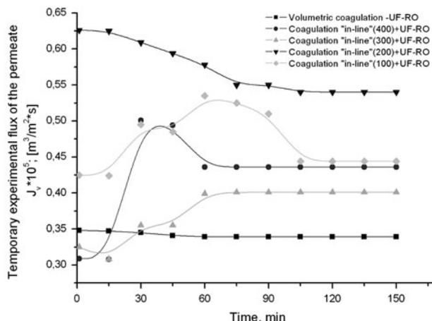
Fig. 3. Dependence of temporary experimental volumetric fluxes on time treatment coke-making reverse osmosis process.
