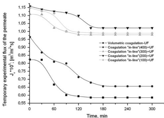
Fig. 2. The dependence of the experimental temporary permeate flux on the time of coke plant wastewater low-pressure membrane filtration.
