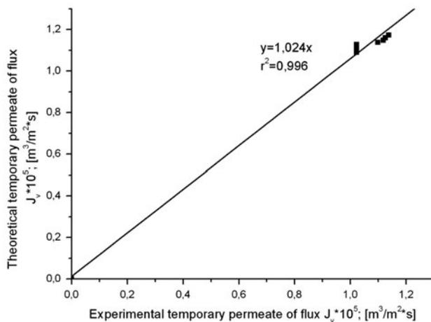
Fig. 4. The graphic comparison of temporary average fluxes of permeate with temporary theoretical obtained in the treatment coke plant wastewater.
