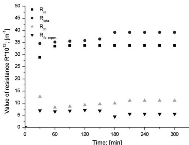
Fig. 6. Comparison of changes in resistance  $R_{total}$ ,  $R_m$ ,  $R_{fm}$ ,  $R_{fo\ exp.}$  polysulfone flat membrane during coke wastewater treatment in hybrid system.
