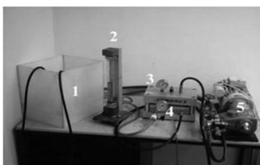
Fig. 1. Photo equipment to conduct the coke wastewater by pressure membrane filtration: 1-tank, 2-rotameter, 3-membrane module, 4-manometer, and 5-high pressure pump.
