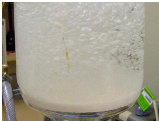
Fig. 3. Photograph of a bubble column containing pure water with an inlet gas flow rate (RT) of 23 L/min at an inlet temperature of 147°C. The column solution temperature was about 45°C.
