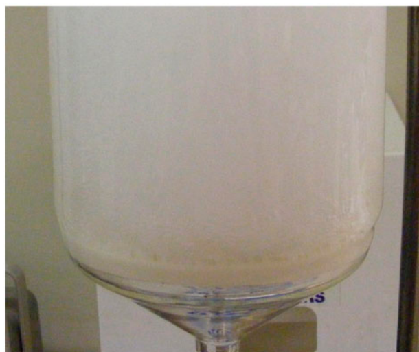
Fig. 4. Photograph of a bubble column containing of 0.5 M NaCl solution with an inlet gas flow rate (RT) of 23 L/min at an inlet temperature of 147°C. The column solution temperature was about 45°C.
