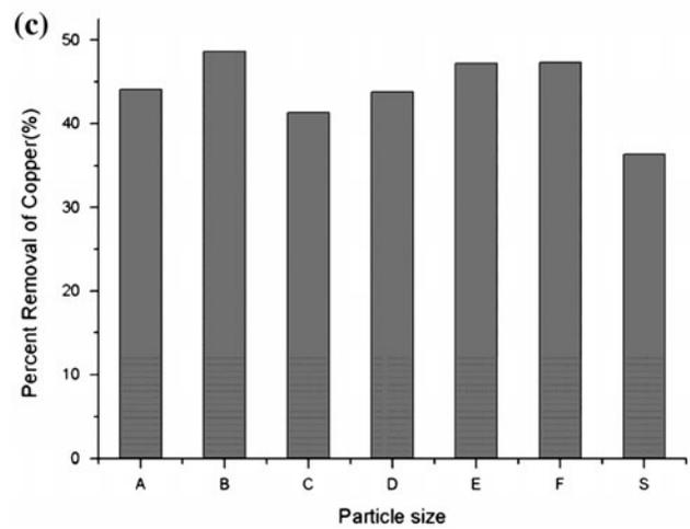
Fig. 10. Effect of partial size on uptake of (a) Pb(II), (b) Cd(II) and (c) Cu(II) by fruiting bodies and spores of *O. radicata* (biosorbent dosage = 5 g/L, initial metal concentration = 100 mg/L, contact time = 3 h and pH 5.0).
