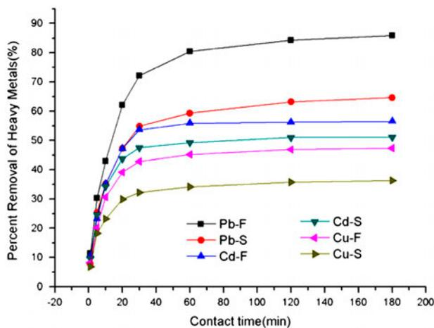
Fig. 4. Effect of contact time on sorption of Pb(II), Cd(II) and Cu(II) by fruiting bodies and spores of *O. radicata* (initial metal concentration = 100 mg/L, biomass dosage = 5 g/L and pH 4.0).
