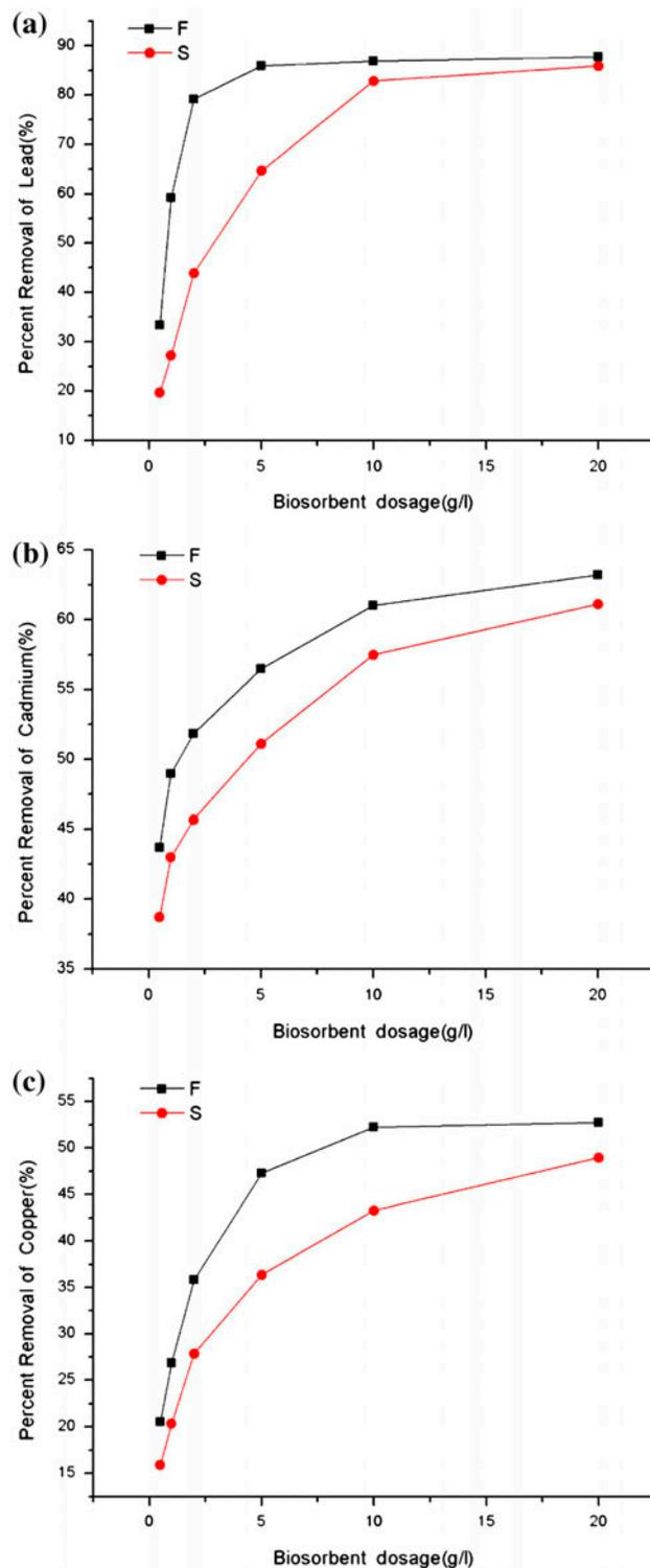
Fig. 3. Effect of biosorbent dosage on sorption of (a) Pb(II), (b) Cd(II) and (c) Cu(II) by fruiting bodies and spores of *O. radicata* (initial metal concentration = 100 mg/L, pH 4.0 and contact time = 3 h).
