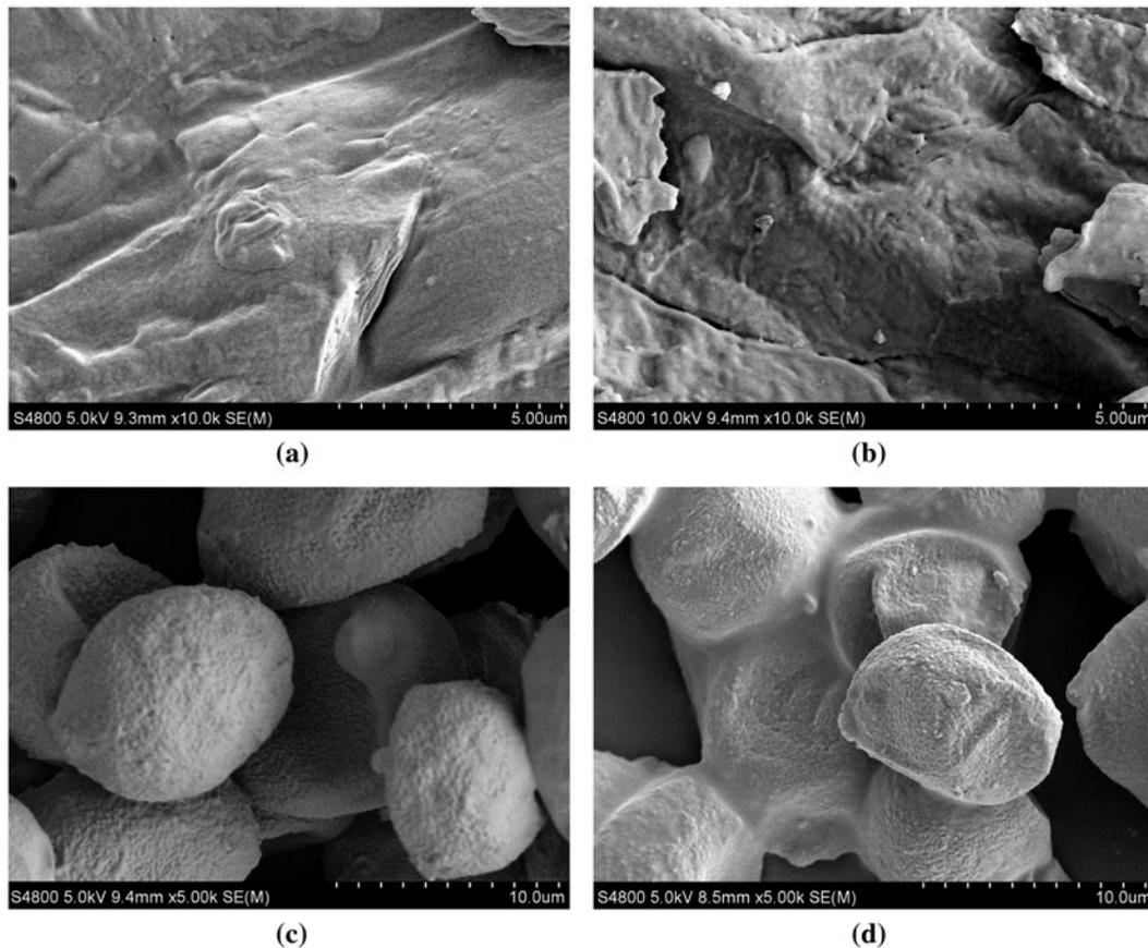
Fig. 11. SEM images of fruiting bodies and spores of *O. radicata* biomass before and after biosorption. (a) Fruiting bodies and (c) spores before Pb(II) biosorption, (b) fruiting bodies and (d) spores after Pb(II) biosorption.
