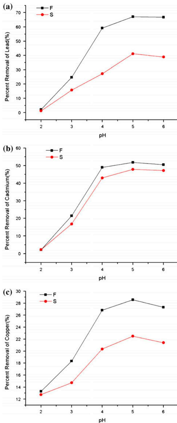
Fig. 2. Effect of pH on sorption of (a) Pb(II), (b) Cd(II) and (c) Cu(II) by fruiting bodies and spores of *O. radicata* (initial metal concentration = 100 mg/L, biosorbent dosage = 1 g/L and contact time = 3 h).
