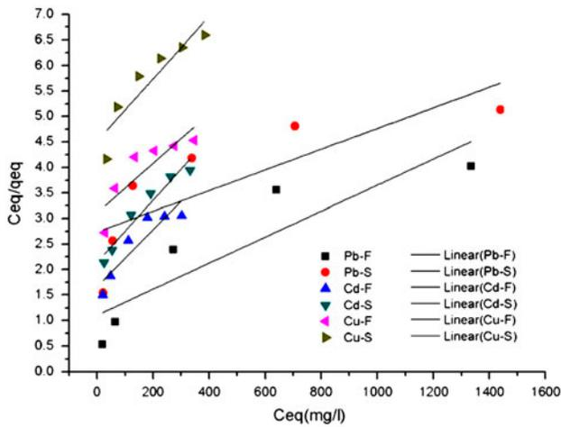
Fig. 8. Langmuir isotherm plots for the biosorption of Pb(II), Cd(II) and Cu(II) by fruiting bodies and spores of *O. radicata*.
