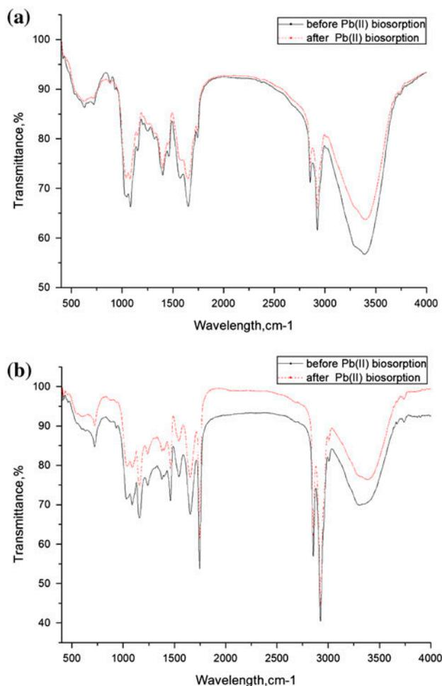
Fig. 13. FT-IR spectrum of unloaded and Pb(II)-loaded biomass (a) fruiting bodies of *O. radicata* biomass and (b) spores of *O. radicata* biomass.
