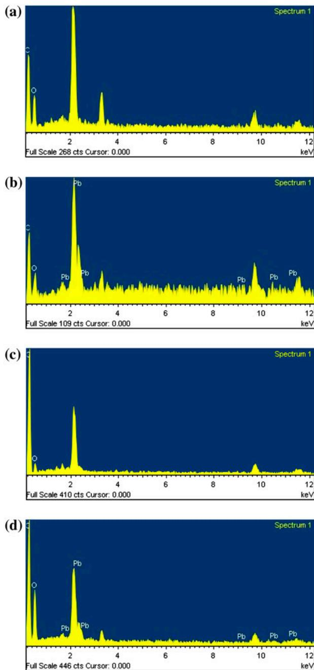
Fig. 12. EDS images of fruiting bodies and spores of *O. radicata* biomass before and after biosorption. (a) Fruiting bodies and (c) spores before Pb(II) biosorption, (b) fruiting bodies and (d) spores after Pb(II) biosorption.
