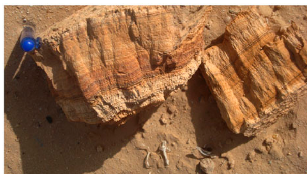
Fig. 6. A sample of tartar deposited in the conduct of the network of Touggourt (photo 2010).
