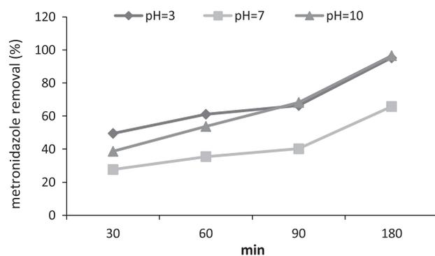
Fig. 10. Effect of pH variation on MNZ removal.
