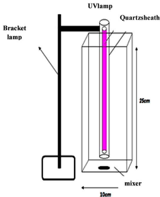
Fig. 5. Schematic of photocatalytic reactor.
