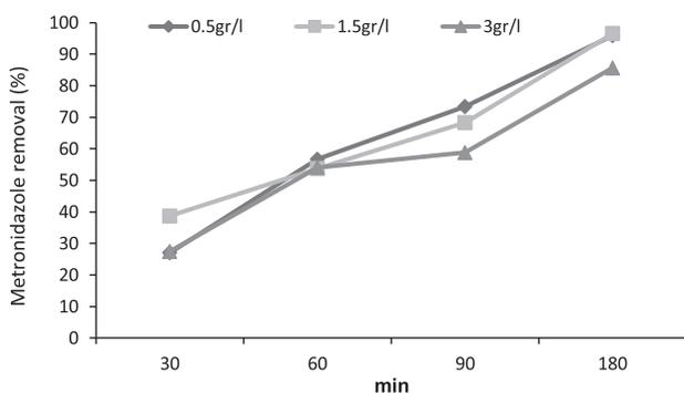
Fig. 8. Effects of variations in nano-ZnO concentration on the removal of MNZ.
