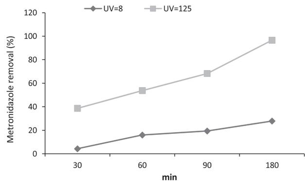
Fig. 6. Removal efficiency of MNZ with radiation intensity 8, 125 W in nano-ZnO/UV process.
