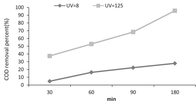
Fig. 7. Removal efficiency of COD with radiation power 8, 125 W in nano-ZnO/UV process.
