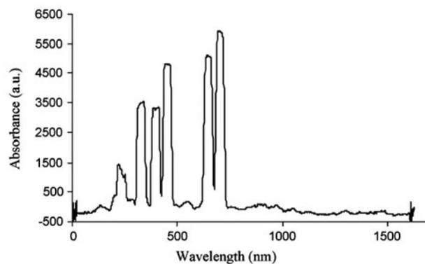
Fig. 4. The spectrum of the UV source that provided by 125 W lamp.
