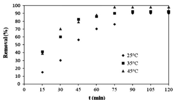
Fig. 9. Effect of temperature on % removal of acyclovir ( $C_0$ : 100 mg/L, PAC: 4 g/L, natural pH, 200 rpm, time: 75 min).
