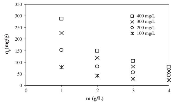
Fig. 7. Effect of PAC dose on acyclovir amount adsorbed (pH: 7, agitation speed: 200 rpm, temp.: 25°C, contact time: 75 min).
