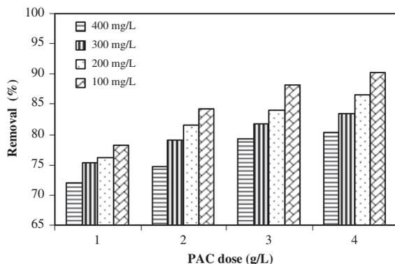
Fig. 6. Effect of PAC dose on % acyclovir removal (pH: 7, agitation speed: 200 rpm, temp.: 25°C, contact time: 75 min).
