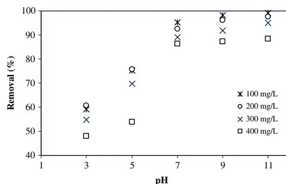
Fig. 10. Effect of pH on adsorption of acyclovir onto powdered activated charcoal ( $C_0$ : 100–400 mg/L, PAC: 4 g/L, natural pH, 200 rpm, 45°C).
