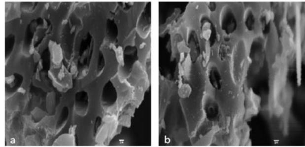
Fig. 5. Scanning electron microscopy images of (a) virgin powdered activated charcoal, (b) acyclovir adsorbed powdered activated charcoal taken at 3,500× magnification, 1 μm scale, 20 kV.
