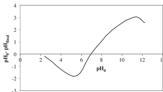
Fig. 2. Determination of  $pH_{zpc}$  of powdered activated charcoal.
