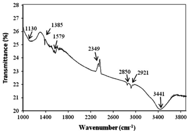
Fig. 3. Fourier transform infrared spectrum of powdered activated charcoal.
