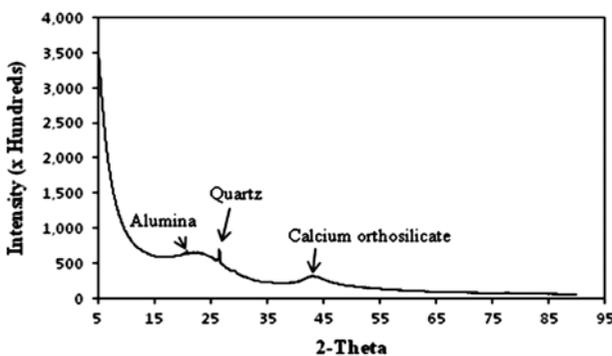
Fig. 4. X-ray diffraction pattern of powdered activated charcoal.
