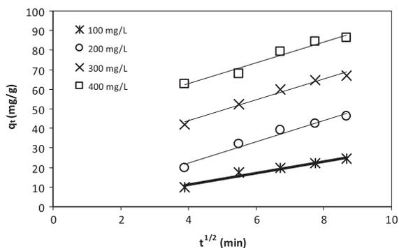
Fig. 11. Intraparticle diffusion plot for acyclovir adsorption onto powdered activated charcoal ( $C_0$ : 100–400 mg/L, PAC dose: 4 g/L, pH: 7, agitation speed: 200 rpm, temp.: 45°C).
