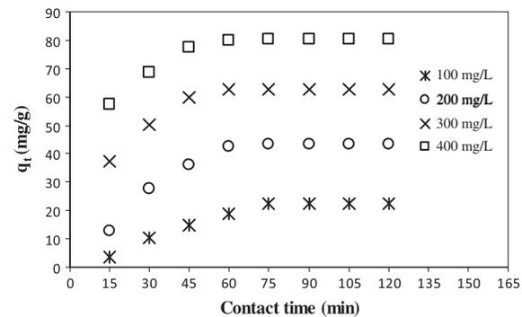
Fig. 8. Amount adsorbed,  $q_t$  (mg/g) of acyclovir vs. contact time (PAC dose: 4 g/L, pH: 7, 200 rpm, temp.: 25°C).
