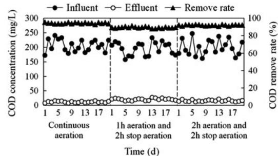
Fig. 6. The comparison of COD removal effect of the continuous operating condition and the intermittent aeration condition.
