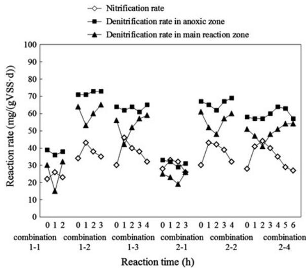
Fig. 5. The changes of nitrification rate and denitrification rate of different combinations of aeration and stop aeration.
