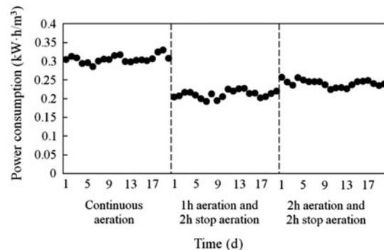
Fig. 10. The comparison of operating power consumption of continuous aeration and intermittent aeration.
