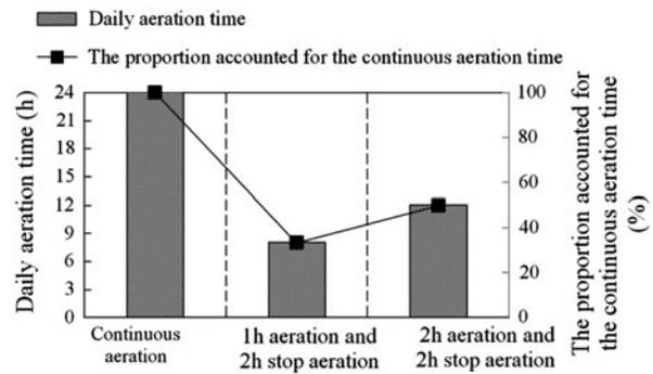
Fig. 9. The comparison of aeration time of continuous aeration and intermittent aeration.
