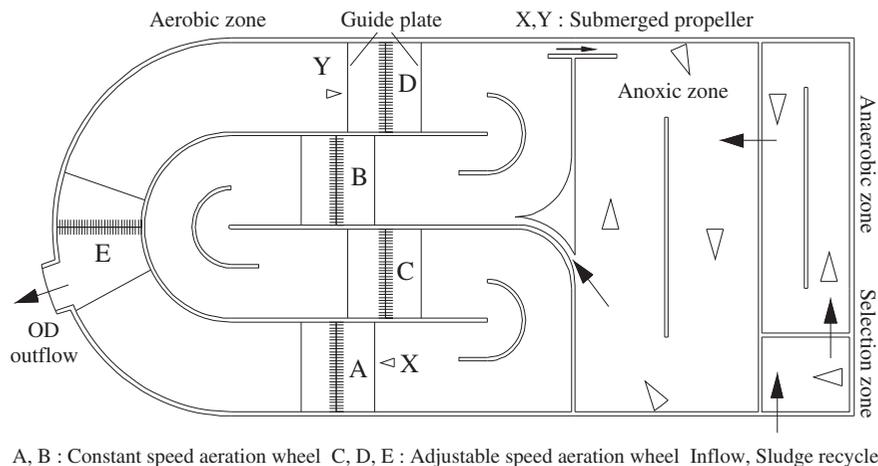
Fig. 1. Layout plan of modified carousel oxidation ditch.
