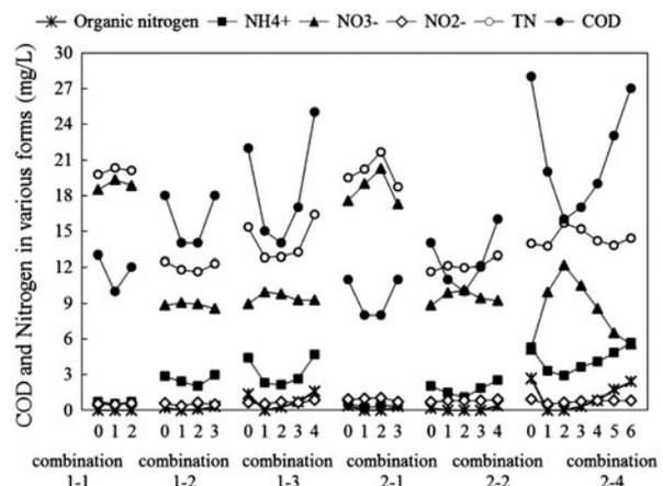
Fig. 4. The changes of effluent COD, organic nitrogen,  $\text{NH}_4^+$ ,  $\text{NO}_3^-$ ,  $\text{NO}_2^-$ , and TN of different combinations of aeration and stop aeration.
