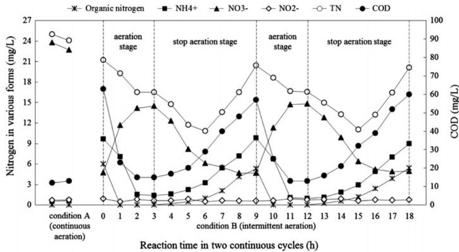
Fig. 2. The changes of effluent COD, organic nitrogen,  $\text{NH}_4^+$ ,  $\text{NO}_3^-$ ,  $\text{NO}_2^-$ , and TN of the system in reaction cycle under the condition A and condition B.
