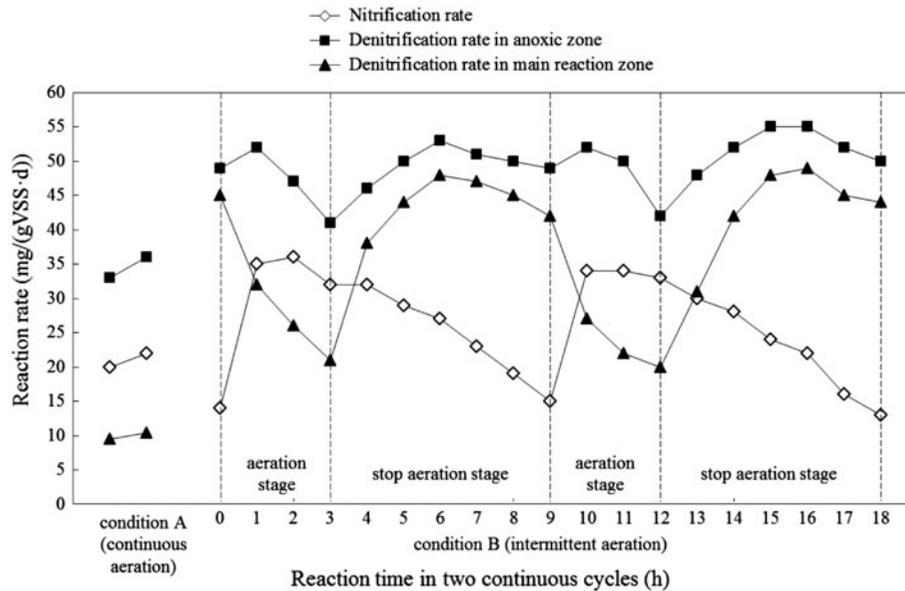
Fig. 3. The changes of nitrification rate and denitrification rate of reaction cycle under the condition A and condition B.
