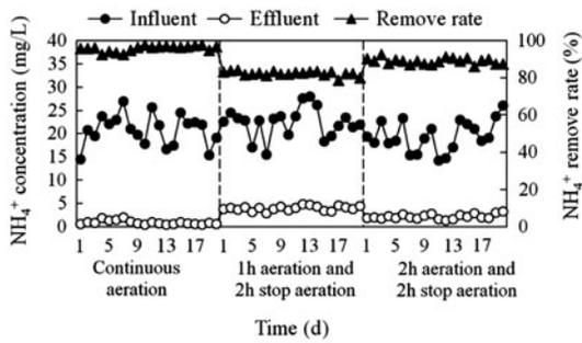
Fig. 7. The comparison of  $\text{NH}_4^+$  removal effect of the continuous operating condition and the intermittent aeration condition.
