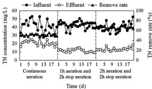
Fig. 8. The comparison of TN removal effect of the continuous operating condition and the intermittent aeration condition.
