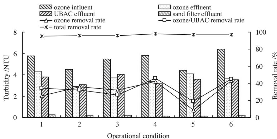
Fig. 8. Effect of operational conditions on turbidity removal in November.
