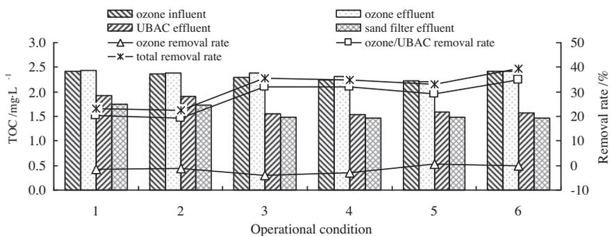
Fig. 4. Effect of operational conditions on TOC removal in November.
