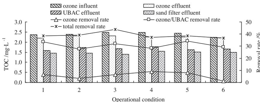
Fig. 5. Effect of operational conditions on TOC removal in May.
