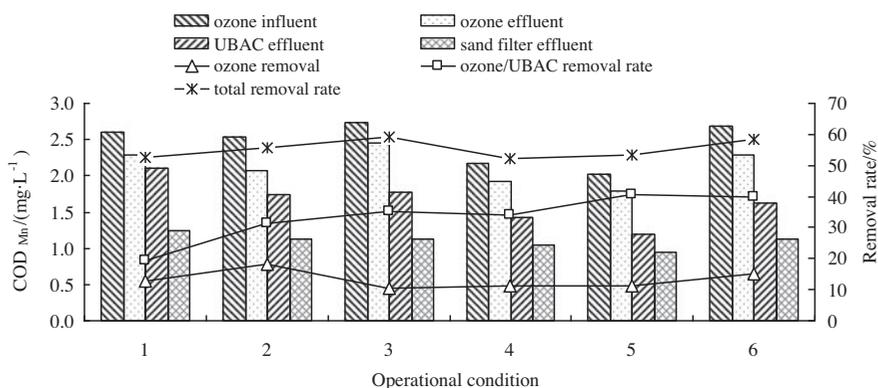
Fig. 3. Effect of operational conditions on COD<sub>Mn</sub> removal in May.
