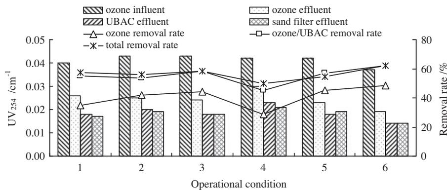
Fig. 7. Effect of operational conditions on  $UV_{254}$  removal in May.
