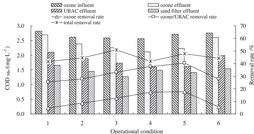
Fig. 2. Effect of operational conditions on COD<sub>Mn</sub> removal in November.
