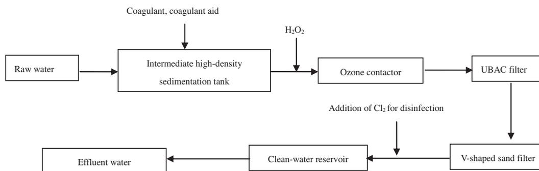
Fig. 1. Process flow of the water treatment plant.
