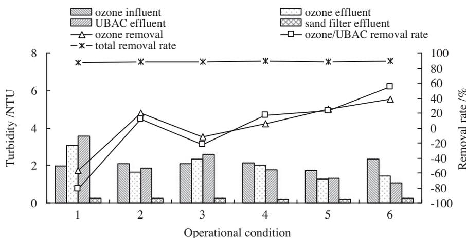
Fig. 9. Effect of operational conditions on turbidity removal in May.
