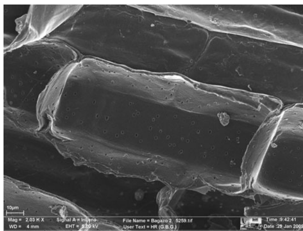
Fig. 2. Scanning electron micrographs of SCB. (Mag: 2.03 KX. EHT: 5.00 kV. WD = 4 mm).
