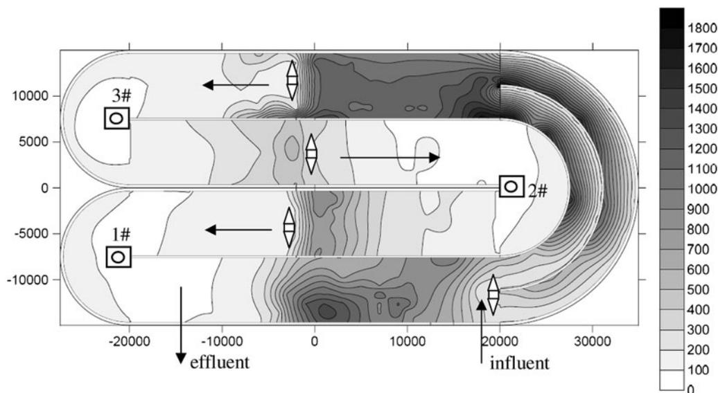
Fig. 4. Sludge deposition height distribution (unit: mm).
