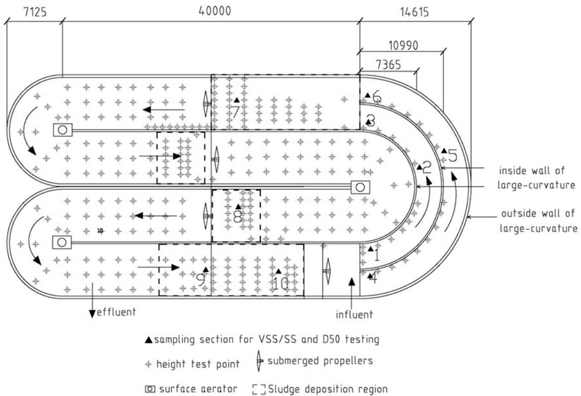
Fig. 2. Schematic diagram of sampling locations (unit: mm).
