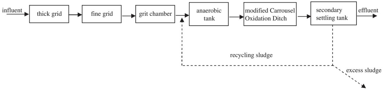
Fig. 1. Schematic of WWTP.
