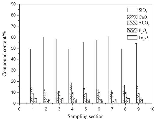
Fig. 11. Inorganic component characterization of deposited sludge.
