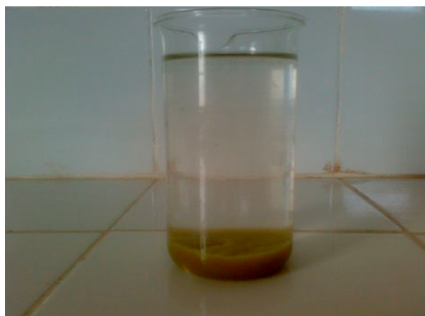
Fig. 6. Industrial wastewater treated by the clay of Maghnia.
