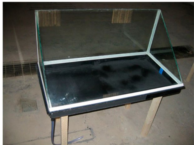
Fig. 2. Single slope solar still with 35° glass tilt angle.
