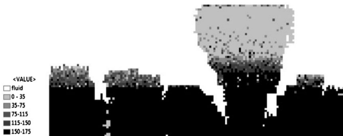
Fig. 1. Map of E_{comp} throughout the biofilm for an UMCCA sample. Values in the legend are in Pa. The conditions relevant to the development of this sample appear in Lapidou and Rittmann [9]. Figure is adapted from Lapidou et al. [19].
